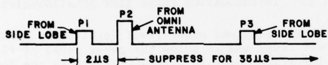
AIRCRAFT A. SIGNALS RECEIVED BY TRANSPONDER (REPLY SUPPRESSED)
