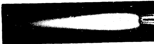
FIG. 38 p = 1 atm d = 0.03 cm 55.6\% \text{ H}_2 v_0 = 9.7 cm 3 /sec \bar{U}_G = 137.5 m/sec Re = 1436
