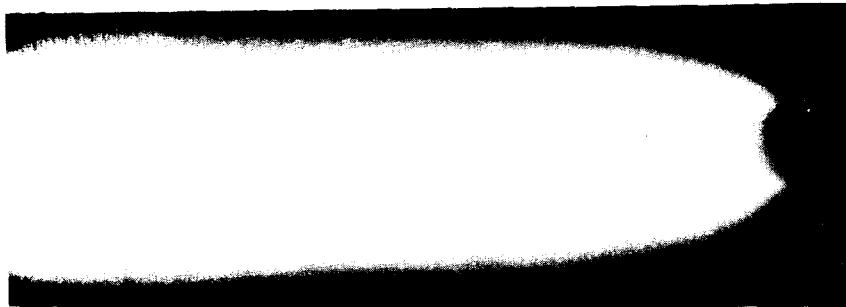
FIG. 27 d = 0.241 cm (water cooled) 71.5 % H_2 v_o = 150 cm^3/sec \bar{U}_G = 33.0 m/sec R_e = 2155
