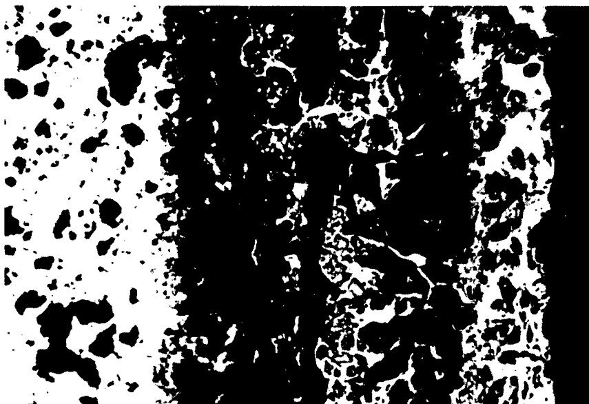
(a) Specimen containing nickel and initially fired at 3200°F. The oxide layer is between the white unoxidized body at the left and the black area on the extreme right which is lucite.
