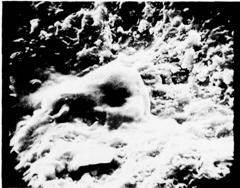
Figure 19. Scanning Electron Micrograph of Fracture Face of R.T. Bend Test Bar of Billet 1937 Material (10% Zyttrite Additive) Featuring Large Grain with Zirconium and Molybdenum Content.
