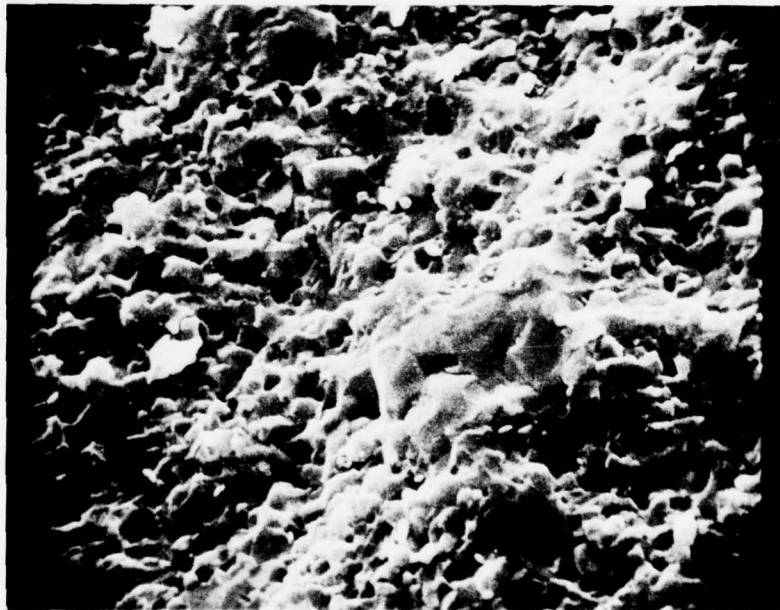
Figure 19. Scanning Electron Micrograph of Fracture Face of R.T. Bend Test Bar of Billet 1937 Material (10% Zyttrite Additive) Featuring Large Grain with Zirconium and Molybdenum Content.
