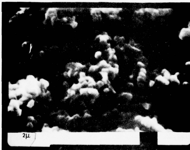
Figure 7. Scanning Electron Micrograph of Blended Silicon Nitride-25 Wt. % Zyttrite Powder.
