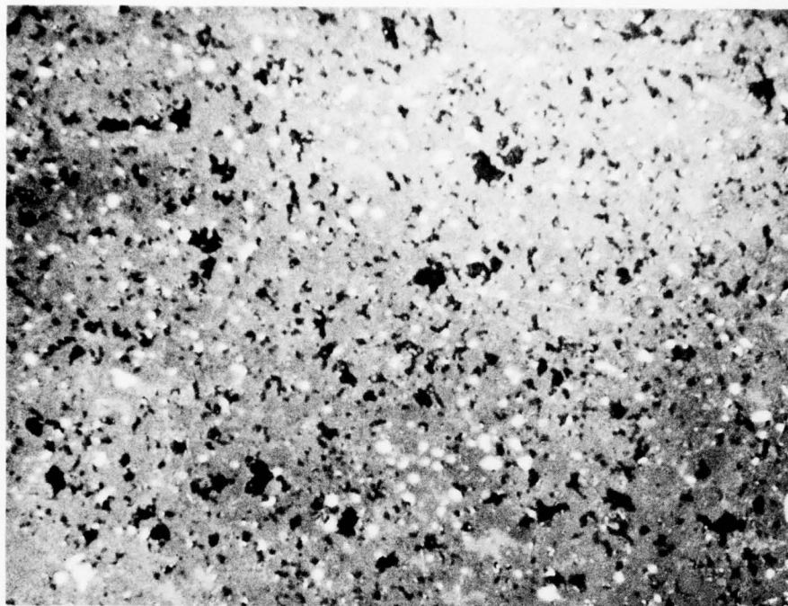
Figure 9. Microphotograph of Cross-Section of Billet 1937 (10% Zyttrite Additive).
