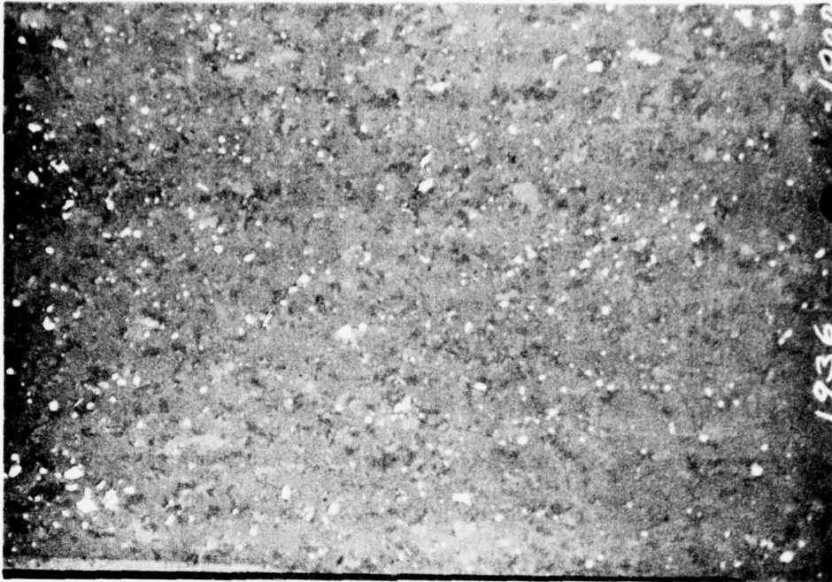
Figure 11. Microphotograph of Cross-Section of Billet 1936 (20% Zyttrite Additive).
