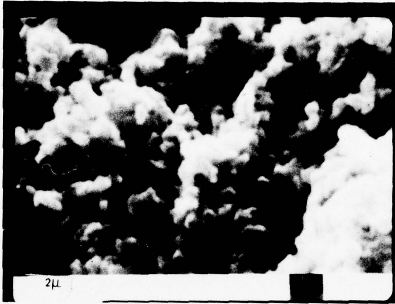
Figure 4. Scanning Electron Micrograph of Blended Silicon Nitride-10 Wt. % Zyttrite Powder.
