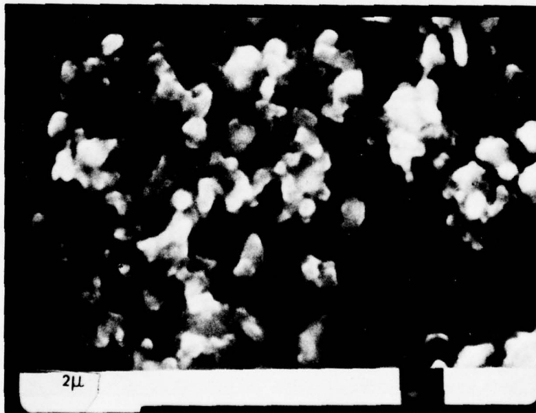
Figure 5. Scanning Electron Micrograph of Blended Silicon Nitride-15 Wt. % Zyttrite Powder.
