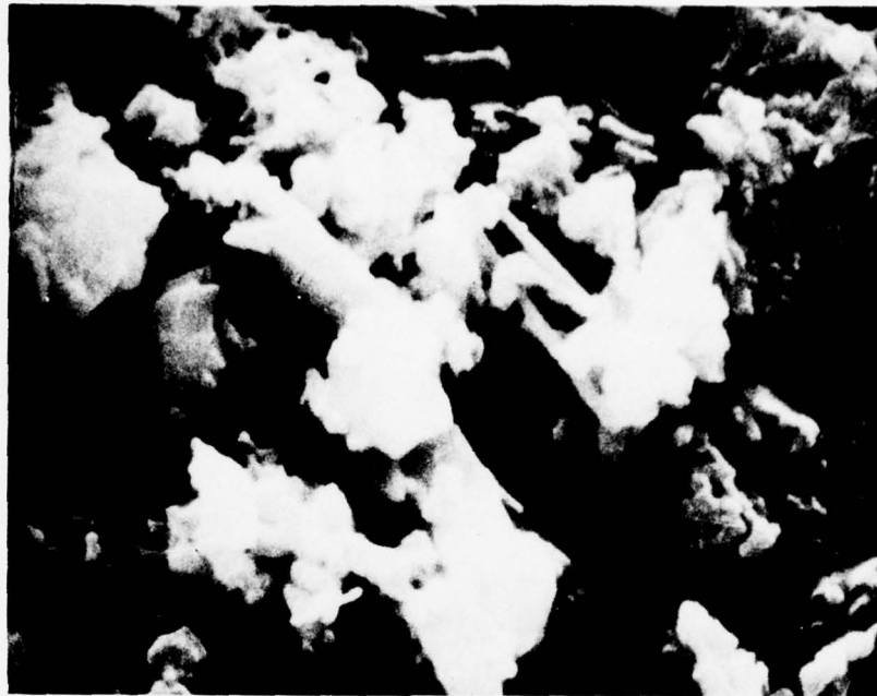
Figure 1. Scanning Electron Micrograph of As-Received Silicon Nitride Powder.
