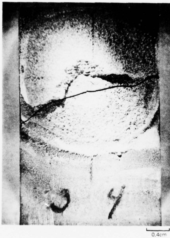
BALLISTIC IMPACT SAMPLE OF NCX-34 \text{Si}_3\text{N}_4 WITH -200 RSSN LAYER (21 V/O Si) AFTER 17.2 JOULE IMPACT
