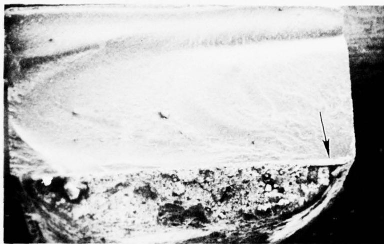
FRACTURE SURFACE OF NC-132 \text{Si}_3\text{N}_4 WITH \sim 325 Å Si LAYER (NITRIDED AT MAXIMUM TEMP. OF 1250°C FOR 24 HRS.)
