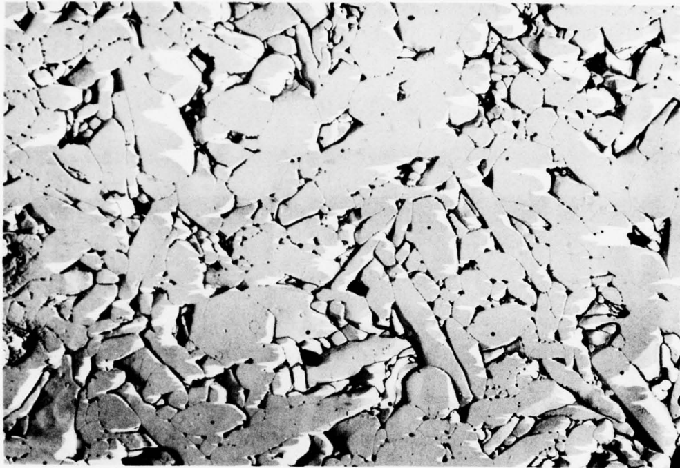
MICROSTRUCTURE OF NC-132 (a) AND NCX-34 (b) HOT-PRESSED \text{Si}_3\text{N}_4 (TEM REPLICA)
