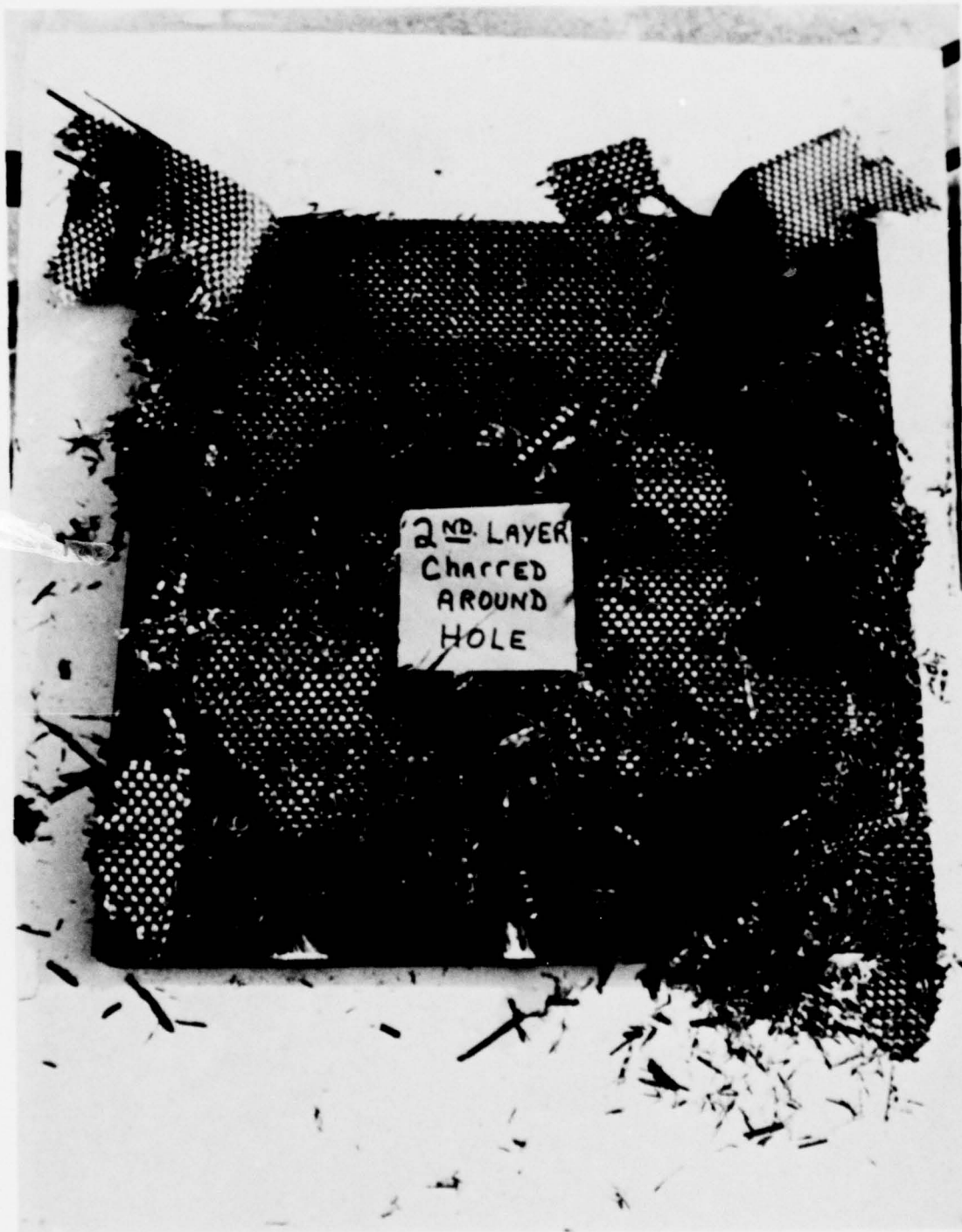
Fiberglass Plate (Of Launcher Tube Simulation Test) Showing Hand Removal Of Second Layer of Char
