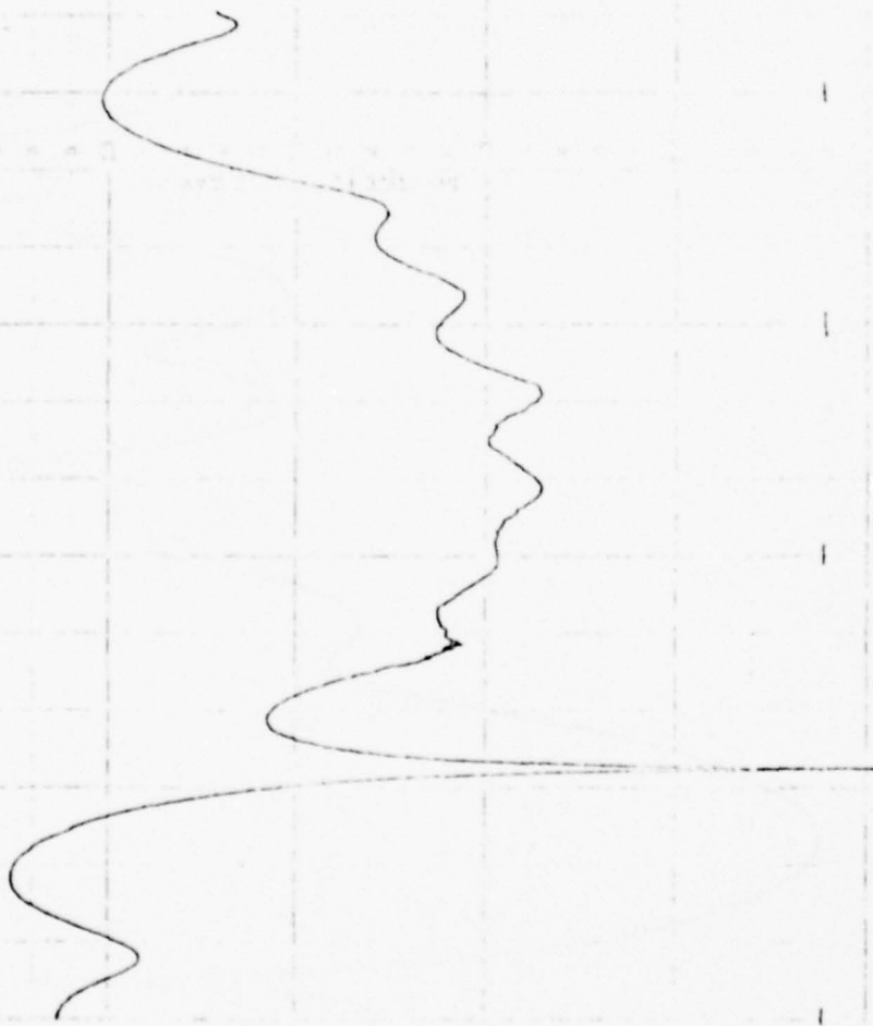
FIGURE 3.34 - SBO PATTERN 38° PHASE ERROR IN BOARD #7
