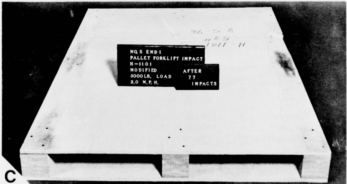
Figure 6.—Typical shear failure patterns of hardboard panels: A. along leading edge, B. along edges of one foot of the load, and C. showing a shear failure in a top deck.
