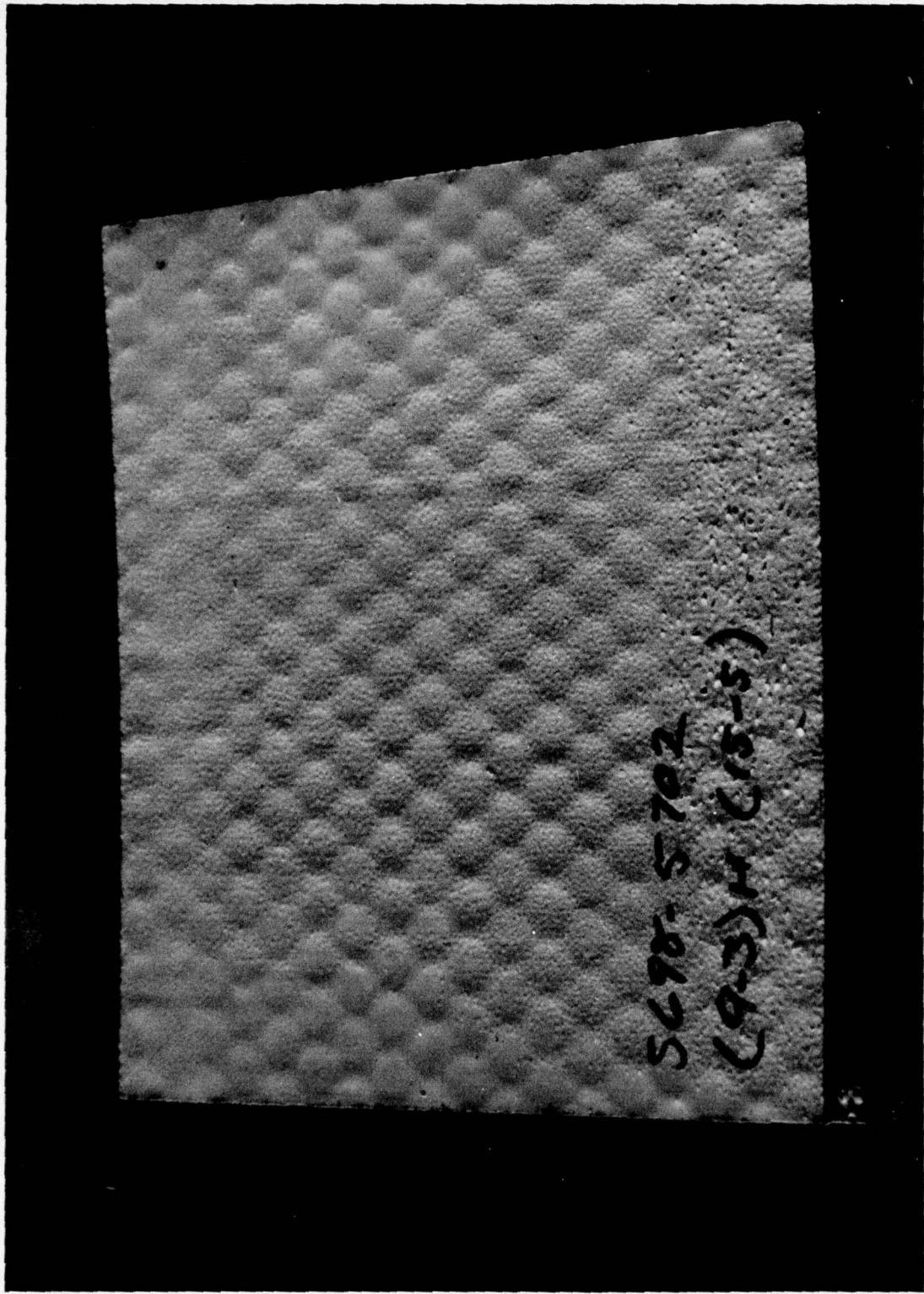
Figure 25. System 9 - 15 cal/cm 2 paint degradation.
