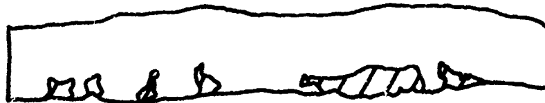
Fracture Surfaces Containing Dross Inclusion Defects. Accompanying Sketches Indicate Extent of Defect as Cross Hatched Areas. Top - Mild, Center - Intermediate, Bottom - Severe. 10X Magnification
