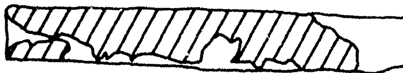
Fracture Surfaces Containing Microshrinkage Defects. Accompanying Sketches Indicate Extent of Defect as Cross Hatched Areas. Top - Mild. Center - Intermediate, Bottom - Severe. 10X Magnification.
