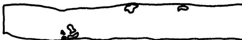
Fracture Surfaces Containing Mold Breakage Inclusion Defects. Accompanying Sketches Indicate Extent of Defect as Cross Hatched Areas. Top - Mild, Center - Intermediate, Bottom - Severe. 10X Magnification.
