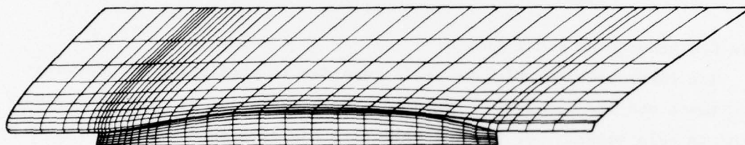
Figure 1 - Typical Panel Arrangement (Dawson, NP 1977)
