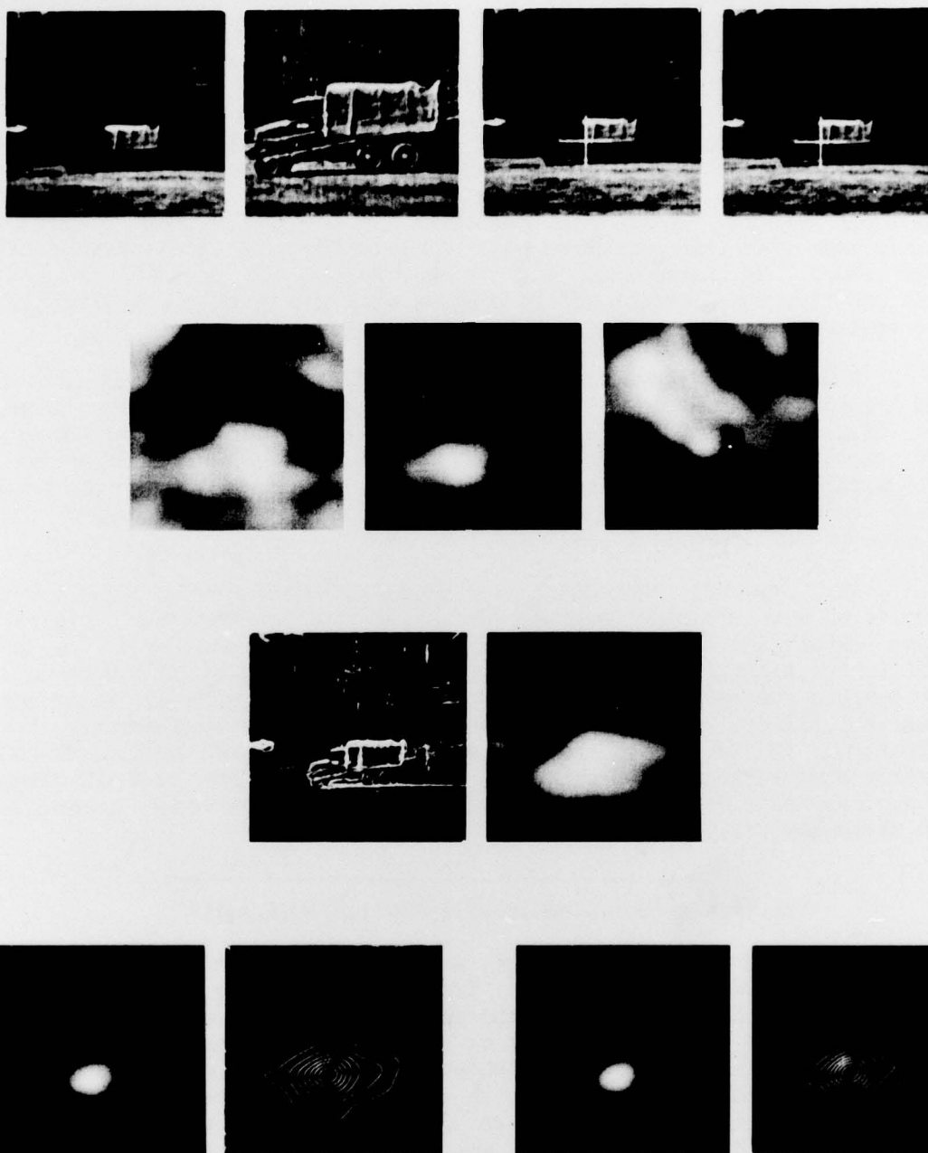
FIGURE 3 - From left to right, the top row shows the original image, the enlarged and enhanced target region, the target designated using the 3 textural features and the target designated using the textural features plus the edge feature. The second row shows the smoothed isotropic texture (reversed polarity), horizontal texture and vertical texture images, whereas the third row shows the edge image before and after smoothing. In the bottom row, the left pair shows the product of the 3 texture images and the right pair the product of the texture images with the smoothed edge image.
