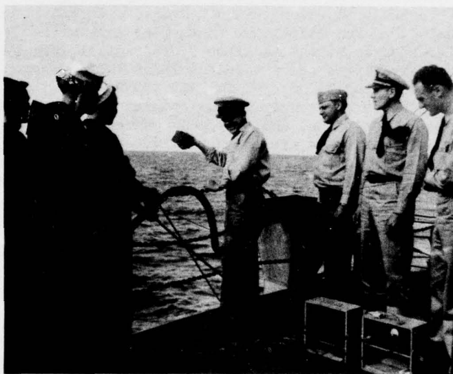
Figure 21. A TNT bomb about to be dropped over the side in a SOFAR test. Hydrophone amplifier in foreground. Seamen are holding lines from the hydrophone, which trail astern of CHILTON (APA-38). ABCR Photo No. 5004-2.
