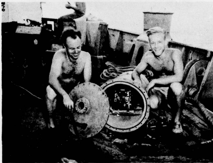
Figure 45. Representatives of Cornell Aeronautical Laboratory with television camera and underwater case. ABCR Photo No. 5082-6.
