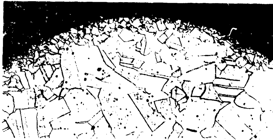
Lot 2 Sealed #188 400X 5% Nital Vendor A 3.5 \mu\text{m} Residual Intergranular Oxide
