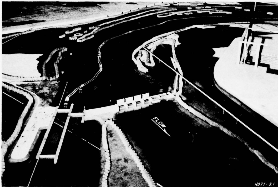
c. Path of 600-ft upbound tow leaving lock showing effects of crosscurrents on head of tow
