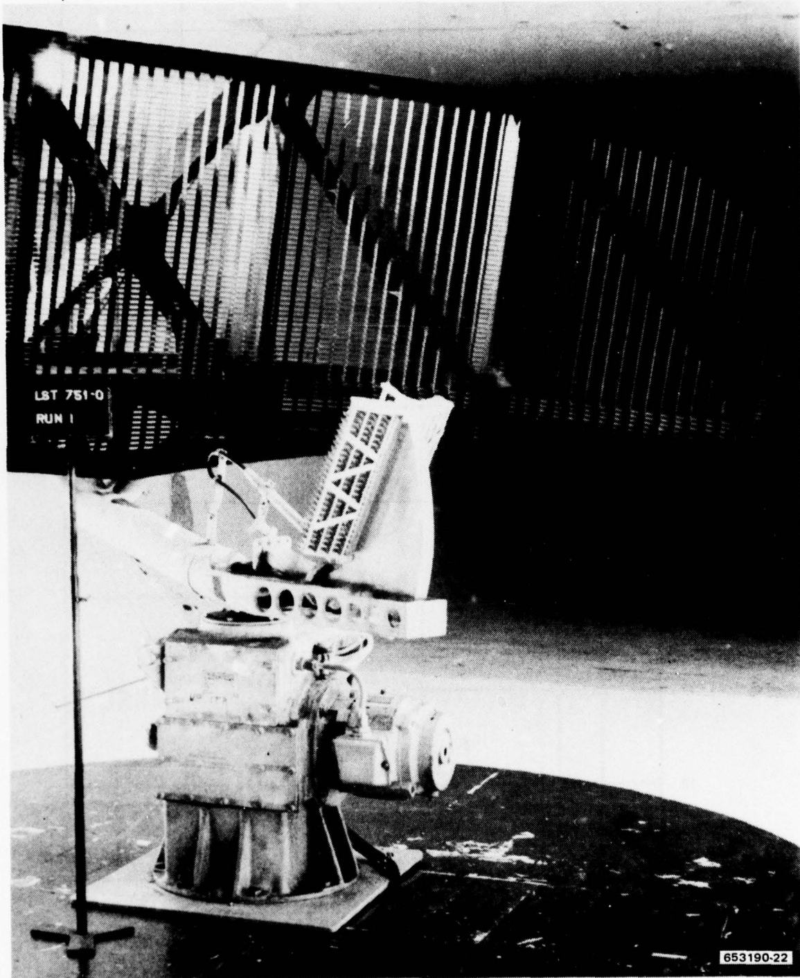
Figure 21. Composite SPS-10 reflector in low-speed wind tunnel - closeup view
