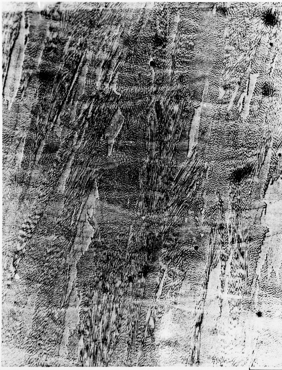
θ FACE NEAR STAINLESS STEEL SUBSTRATE, DISK 1-8, ALLOY 8-12-3
