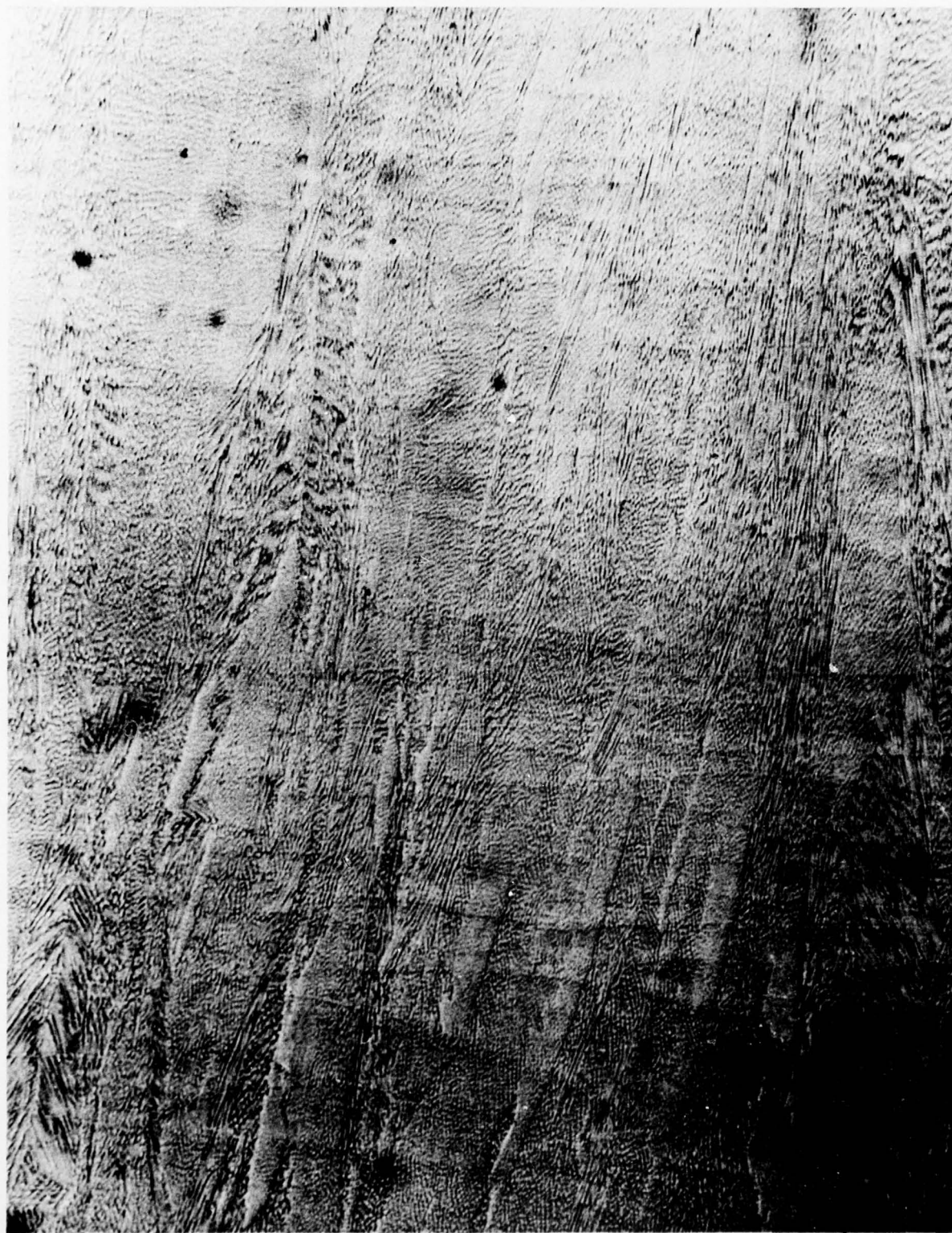
\theta FACE NEAR OUTER SURFACE, DISK 1-8, ALLOY 8-12-3
