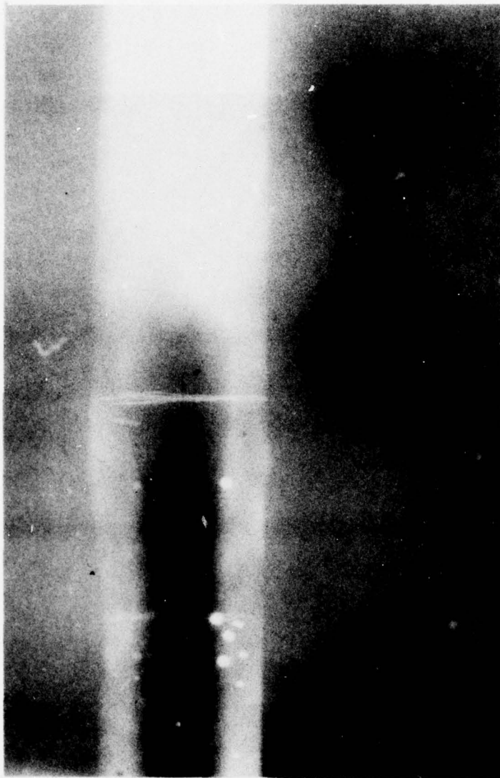
FIGURE 17. RADIOGRAPH OF WELD V-13 0.0 percent Rare-Earth Addition Very Wet Flux
