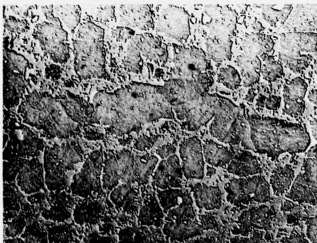
FIGURE 22: \gamma' morphology Alloy 49. Composition (wt.%): as Alloy 44 + 0.15Zr + 0.01B. Extruded bar V159D, Z.A. 2340°F(1280°C)/2.8 iph (7.1 cmph) + 1/2 h/2340°F(1280°C)/AC.
