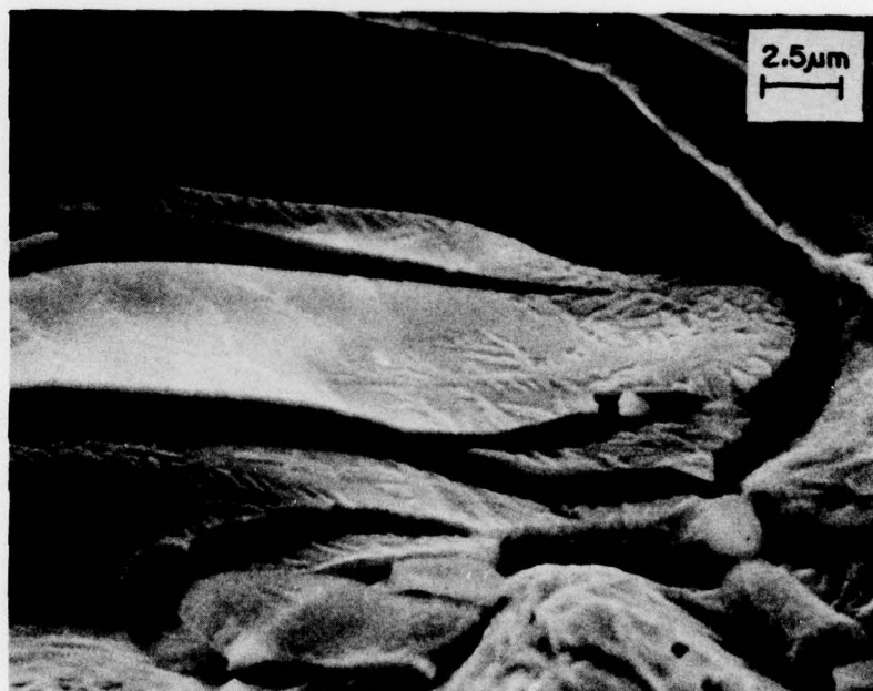
Fig. 13 — Dendritic second phase in silicate platelet. Specimen 0405A.
