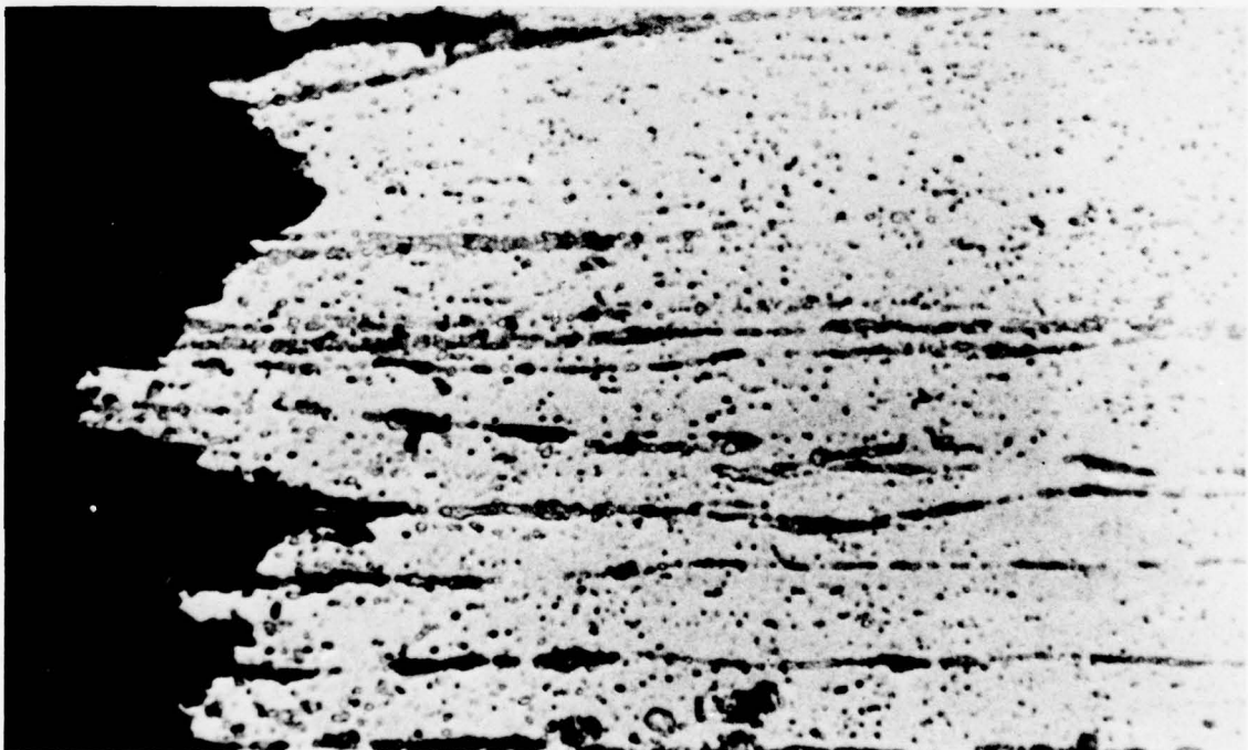
Figure 21. Al-3Li-0.5Fe-0.5Ni consolidated material solution treated 811 K (0.5 h), aged 464 K (8 h)
