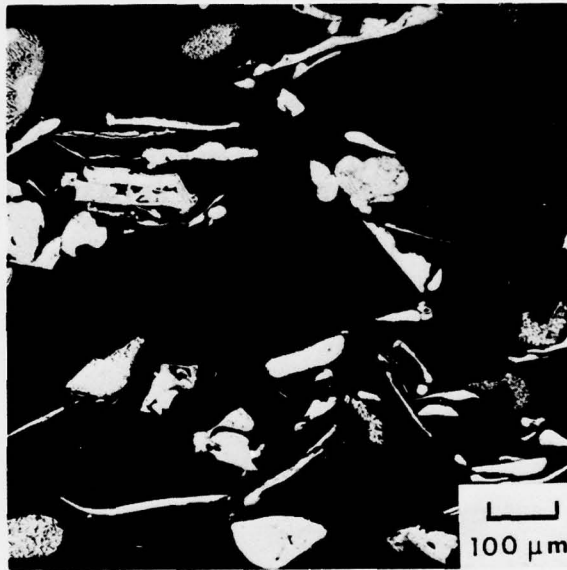
Figure 25. Optical microstructure of particulate in +200 screen fraction of alloy 2.1A (Al-3Fe-3Ni-3Co). Note predominance of in-flight solidified particulate
