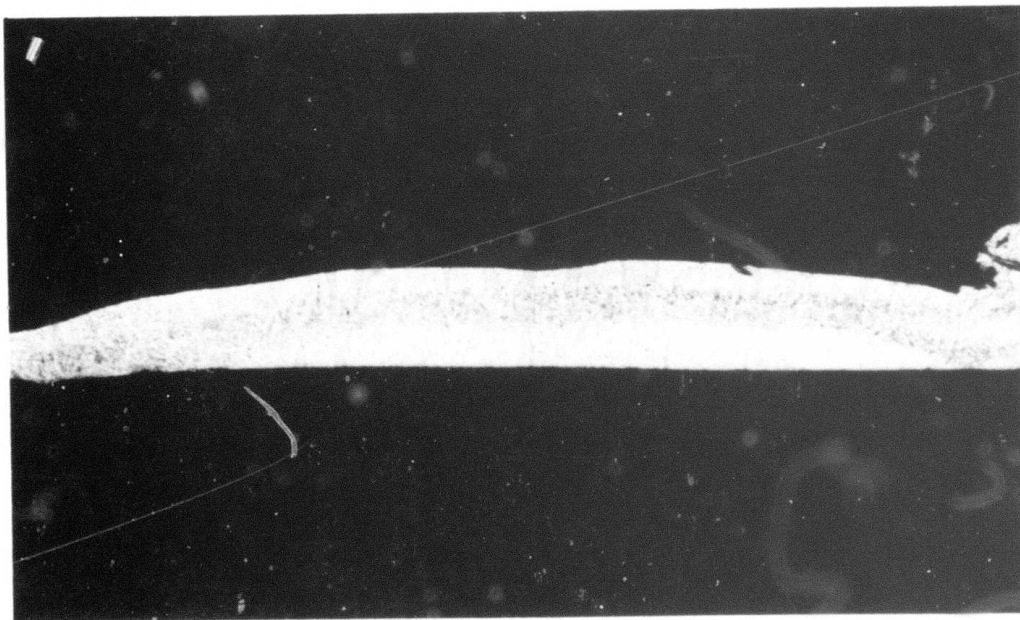
Figure 6. Optical microstructure of alloy 1.1 (Al-4Cu-3Li-0.2Zr), showing typical morphology in the +30 screen fraction: (a) and (b) cellular grain structure in thin flakes, (c) multiple layer flake, (d) dendritic structures
