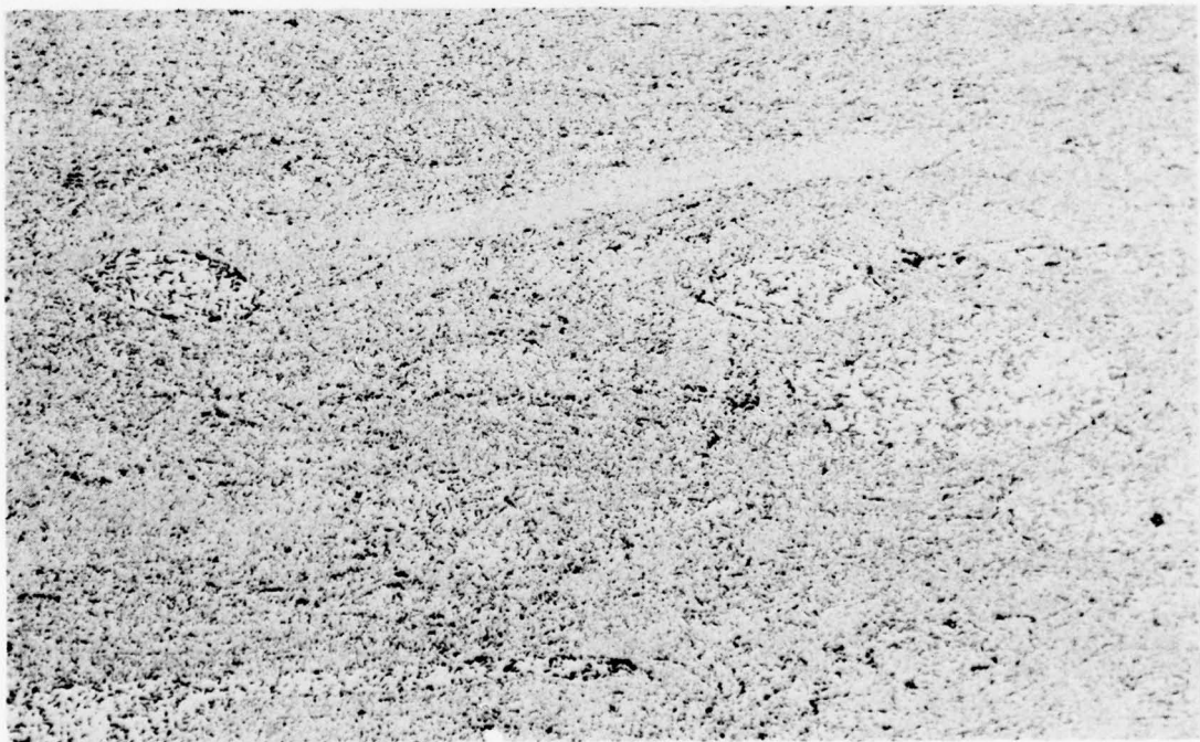
Figure 14. Optical microstructure of alloy 1.1 (Al-4Cu-3Li-0.2Zr) after hot pressing, and extrusion at 700 K (a) longitudinal (b) transverse
