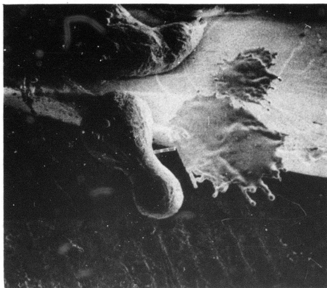
Figure 5. Secondary electron display picture showing adjacent splat and nonsplat particles of alloy 1.1, used for comparison of oxide film thickness
