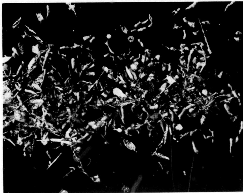
Figure 4. Representative optical micrograph of alloy 1.6 (Al-3Li-1.5Mn) splat, +100 screen fraction
