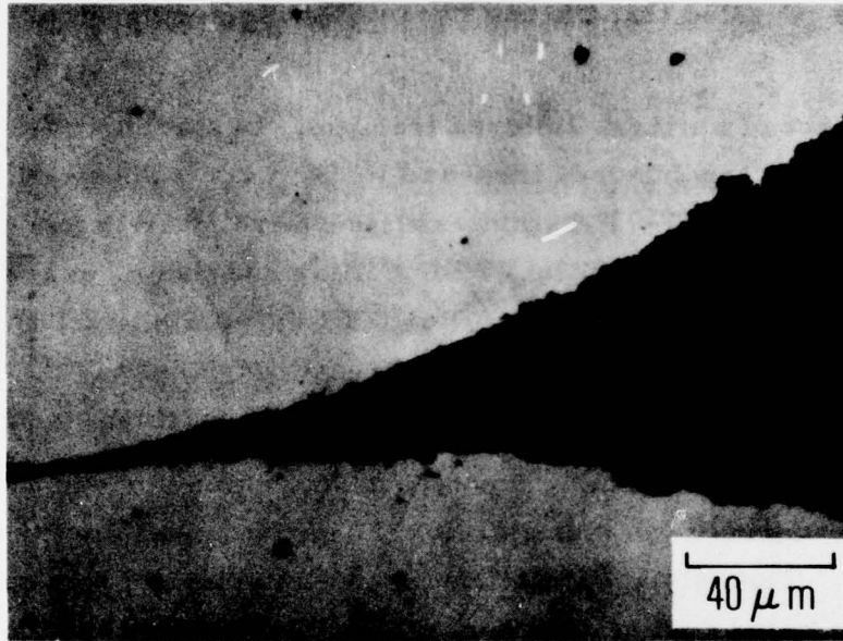
Figure 1. As-Polished Cross-Sectional View of Two Adjacent Coils on a Spring Subjected to a Black Oxide Coating Treatment. Typically, the exposed surface of the wire was rough, whereas unexposed areas near the crevice between adjacent coils were comparatively smooth.
