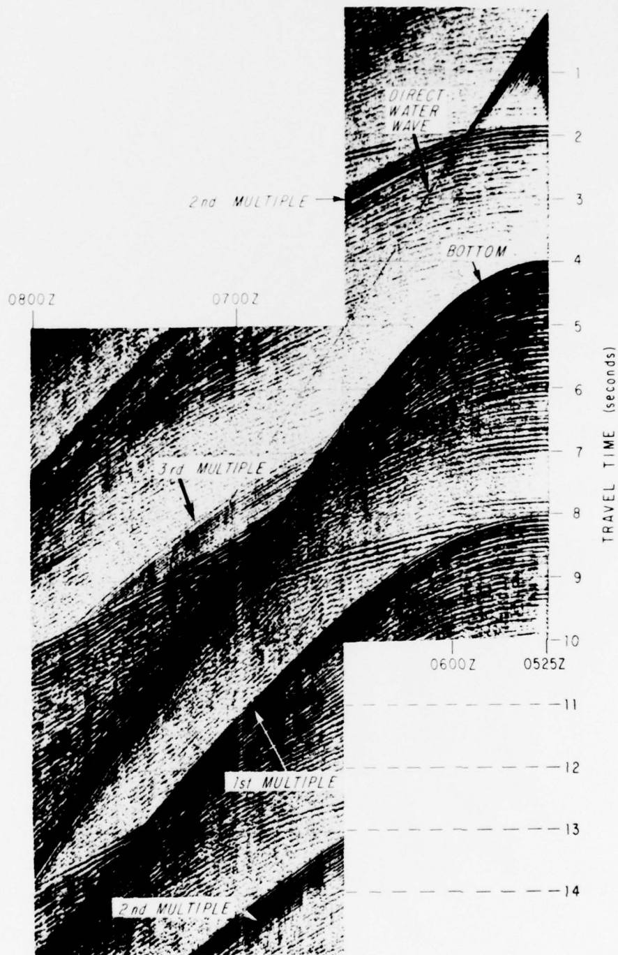
Fig. 3. Wide-angle reflection and refraction record from moored telemetering buoy at station site. Airguns were used as a sound source; ship speed was 4 knots.
