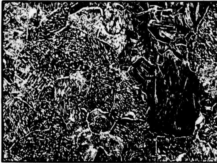
Figure 28. Duplex structure in Ti-17 (250X). (This material, SM-270, was HIP at CSMD at 1600°F and heat-treated without a PCTT)
