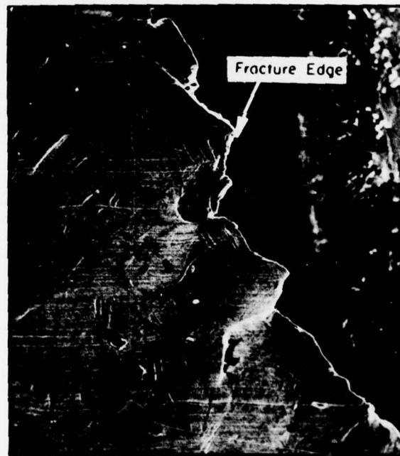
Figure 50. SEM surface images in neckdown area of broken CMRC tensile specimen C4.
