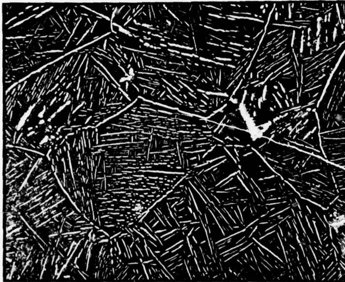
Figure 48. G. E. specimen FT, triplex STA. (G.B. alpha is more broken up and primary alpha more blunted than in the above figure. Both structures are typical for their respective heat treatments - 250X) Etchant: 2%HF - 15%HNO 3
