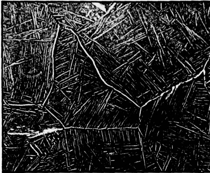
Figure 47. G. E. specimen T1, duplex STA. (G.B. alpha is nearly continuous. Primary alpha needles are sharp. 250X)
