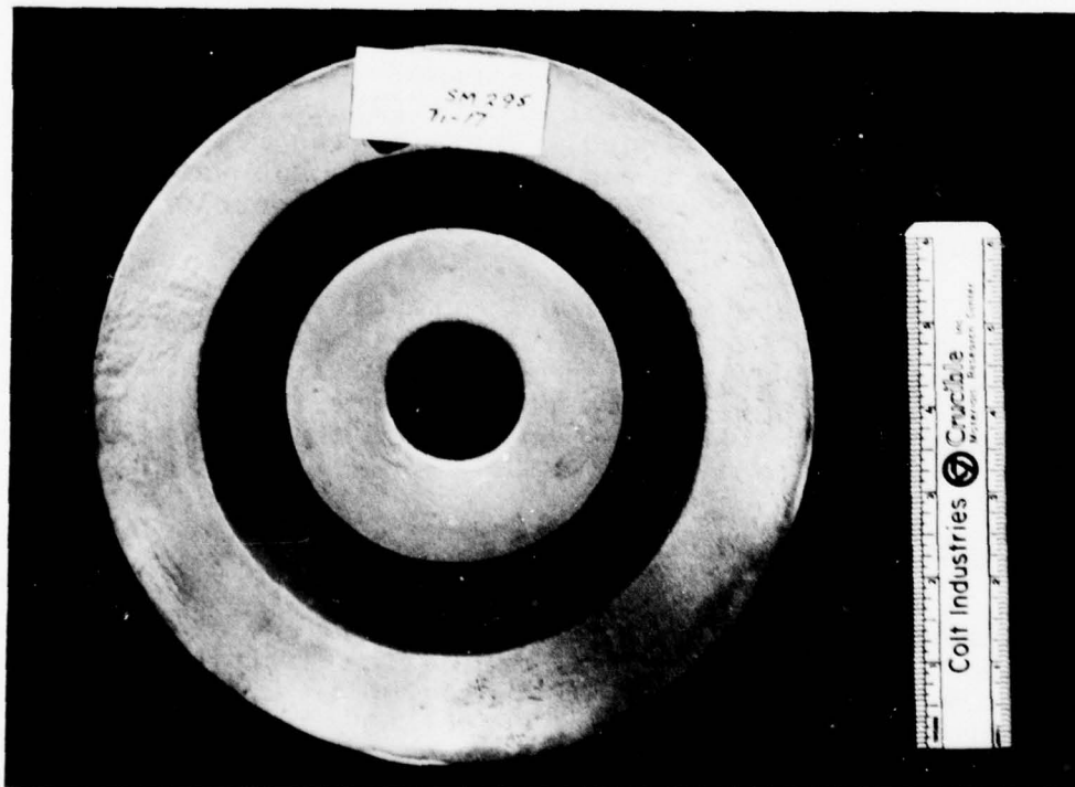
Figure 61. First shape trial on subscale stub shaft.
