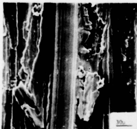
FIGURE 8 Micrograph (SEM) of RMI 5522S, worn surface. ( V=2.1 \text{ ms}^{-1} , \sigma=18.6 \text{ MPa} , N=10^6 cycles).
