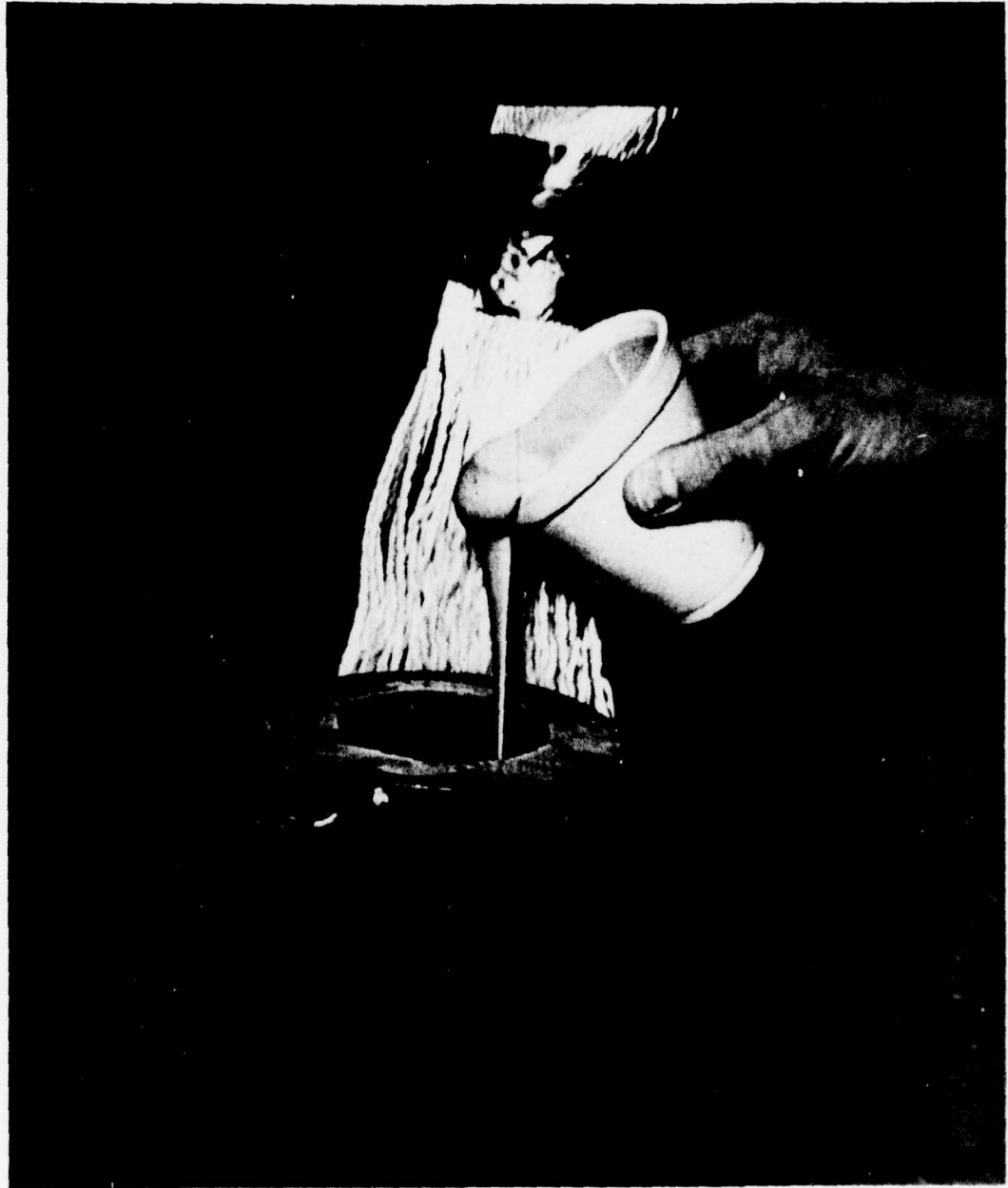
FIGURE 22 PHOTOGRAPHIC REPRESENTATION OF THE SPECIMEN PREPARATION ( POURING EPOXY INTO MOLD )
