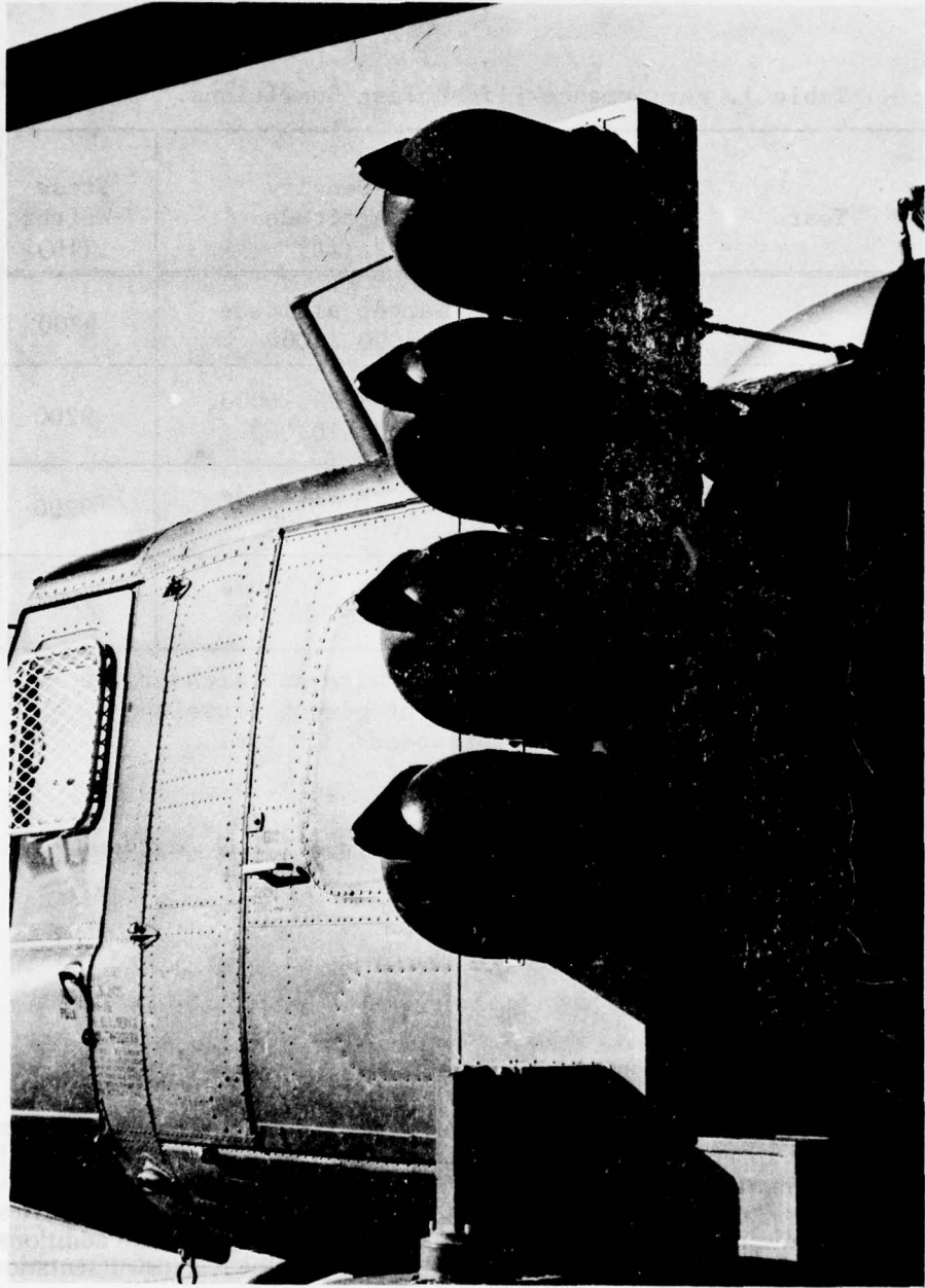
Photo A. JUH-1H with MULTEWS External Boom and Antennae - Left Side.
