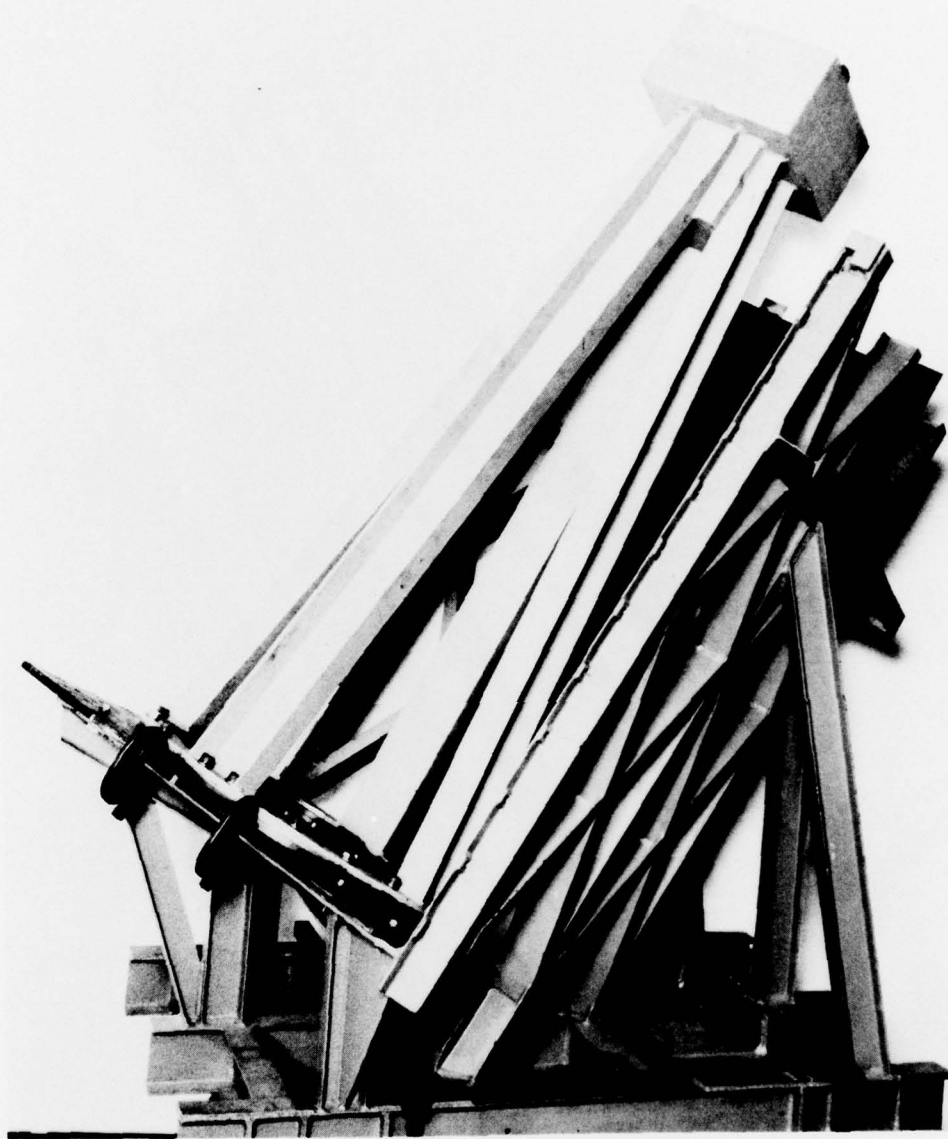
Fig. 22 — Test Structure No. 2 mounted on the MWSM in the 30°-Corner Bulkhead for Inclined Shock
