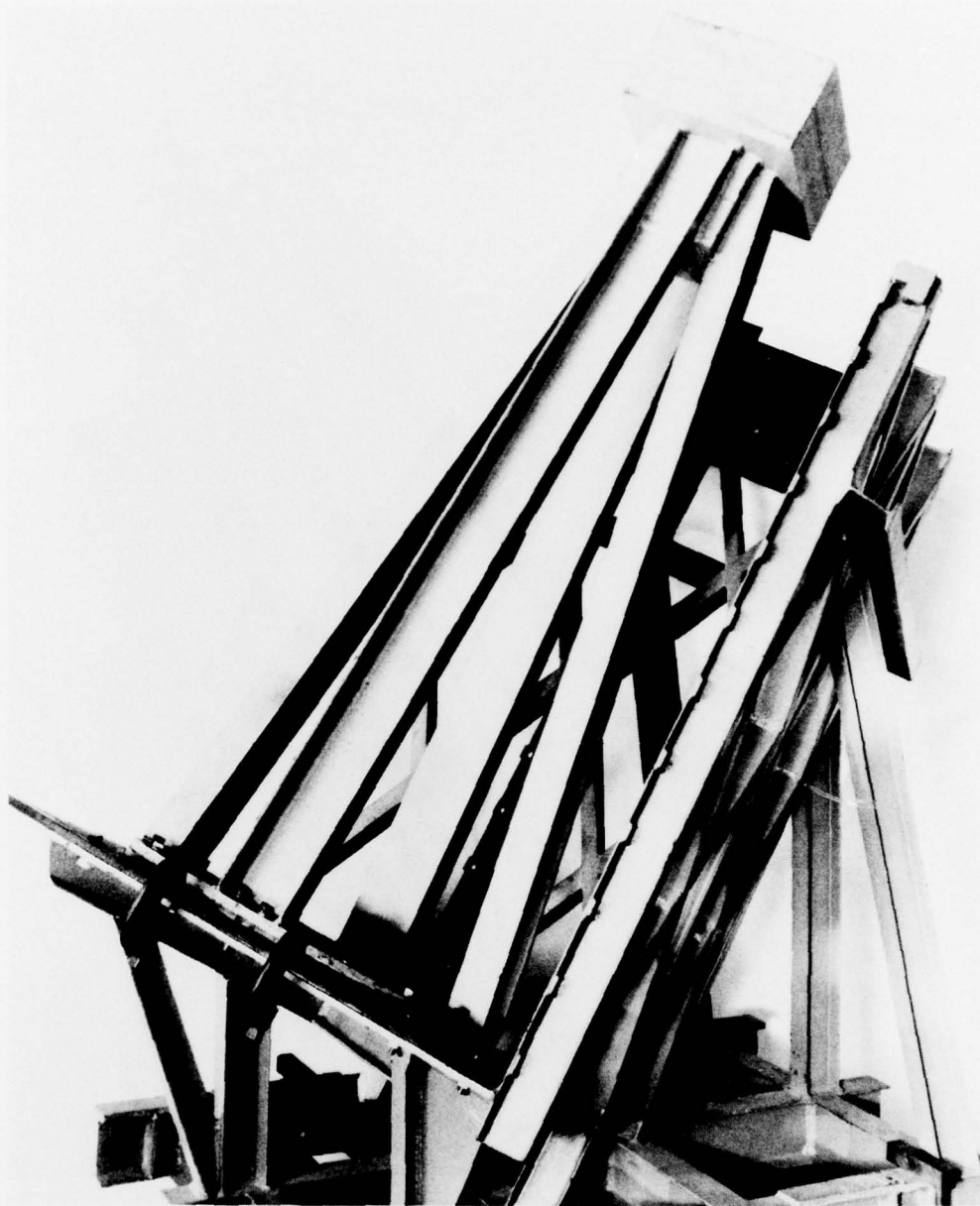
Fig. 21 — Test Structure No. 2 mounted on the MWSM in the 30°-Corner Bulkhead for Inclined Shock
