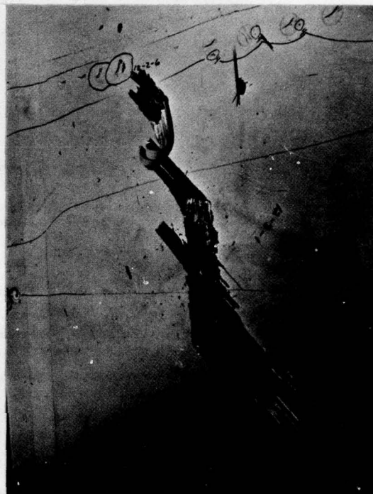
Figure 9 - Closeup of Unprotected B/E After Swept Stroke and Static Restrike Tests
