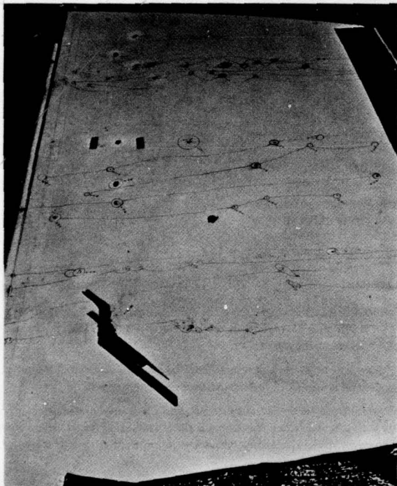
Figure 8 - View of Stub Wing After a Series of Swept Stroke and Static Restrike Tests
