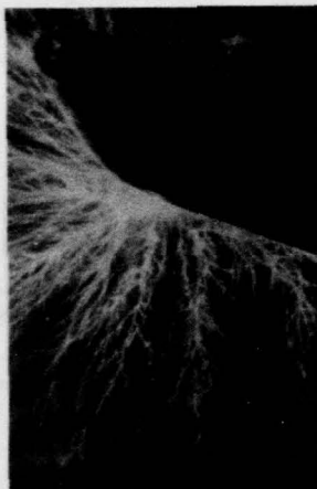
Figure 8b. Streamers on full size NASA re-entrant wingtip vent, with absence of discharges on the fuel vent itself, lower photo, at 8 million volts over 60' to ground.
