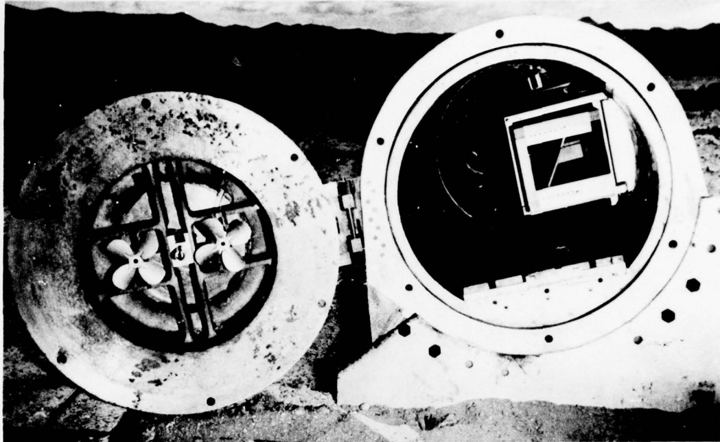
Fig. 2.8 Cylindrical Thermal Exposure Unit with Shutter Housings Open Showing Animal Container, Heater and Ventilation Fans
