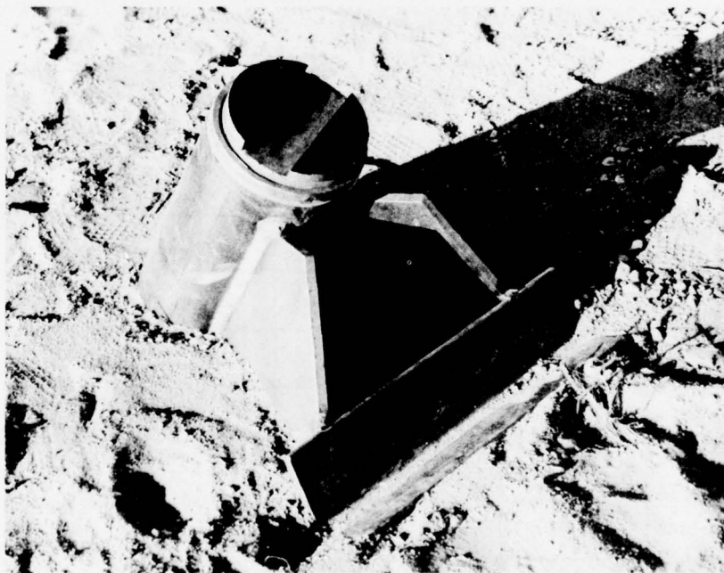
Fig. 3.2 High Level Radiation Exposure Container
