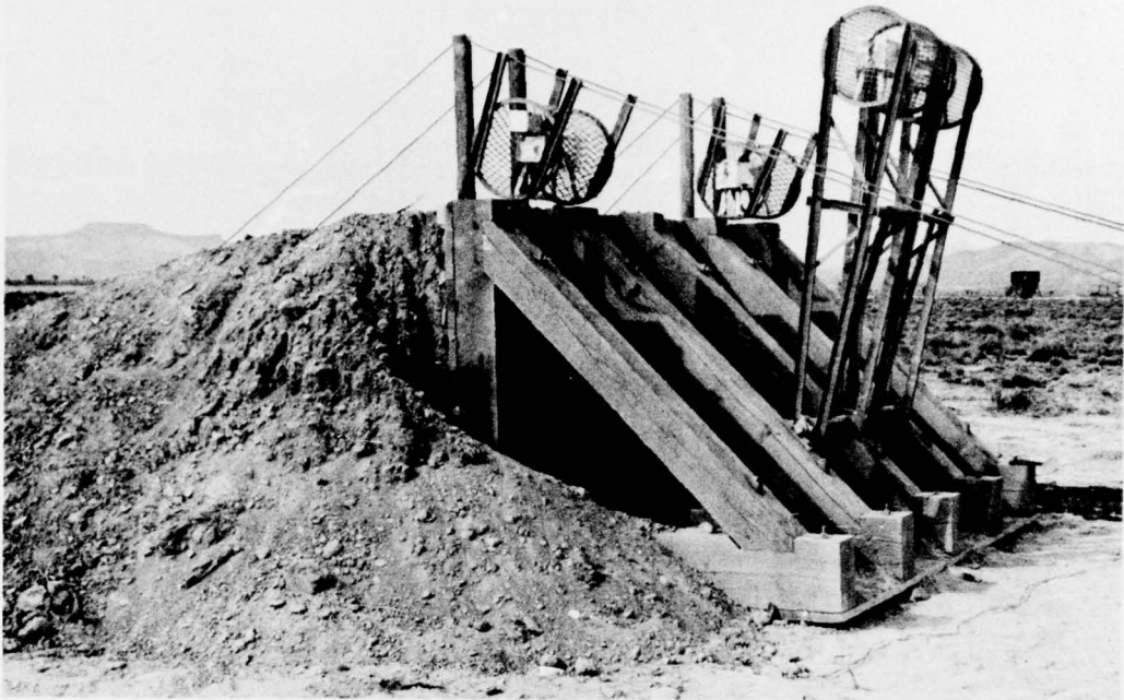
Fig. 1.1 Blast Barrier with Open Mesh Blast Exposure Cage, Side View
