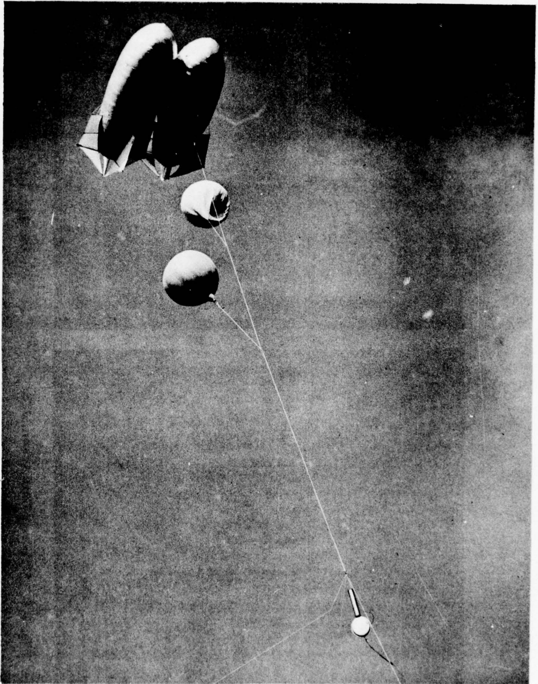
Fig. 2.6 Airborne Unit Supported by Kytoons and Meteorological Balloons
