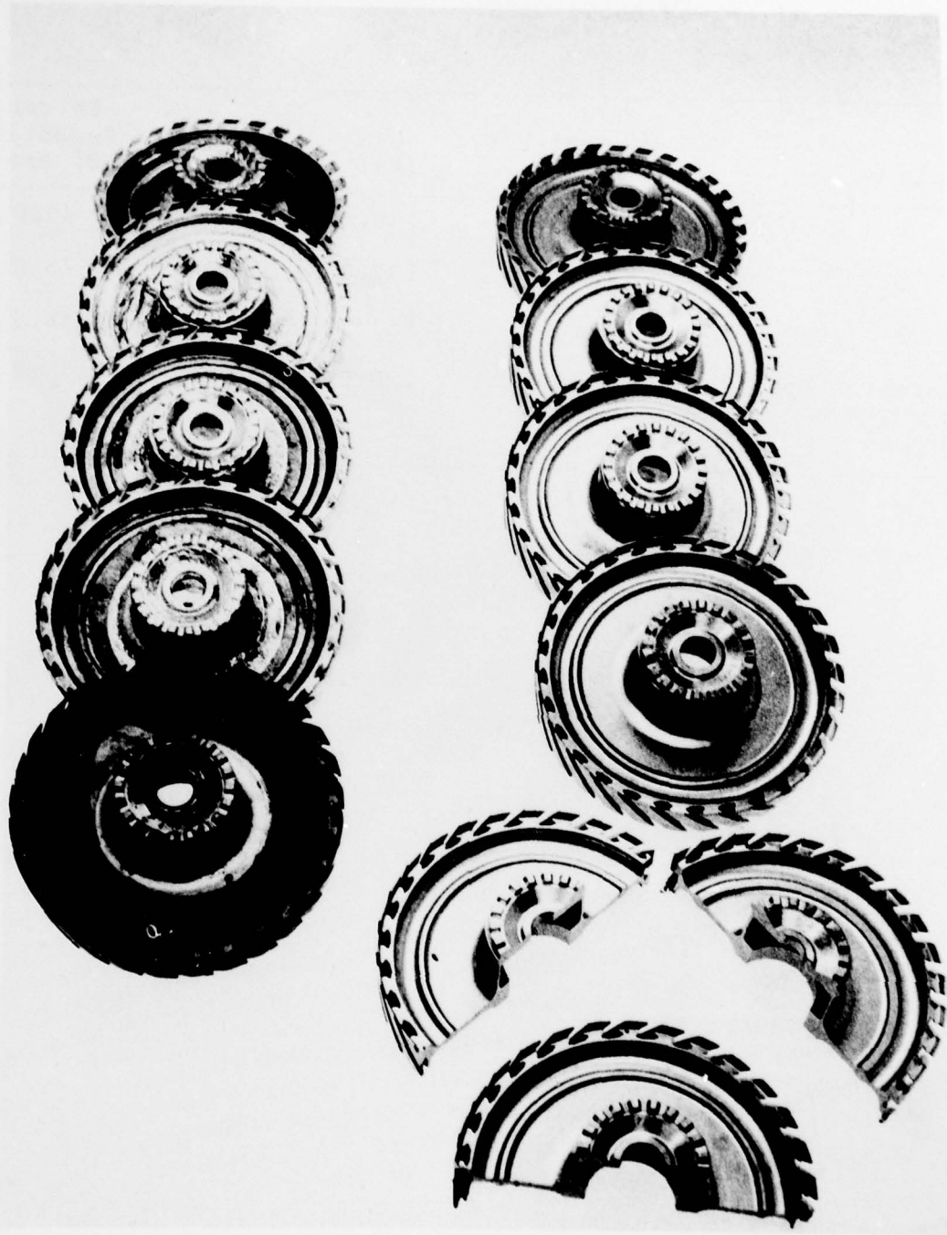
Figure 33. Ti-6Al-4V Alloy Compressor Disks (And Sections) After HIP.
