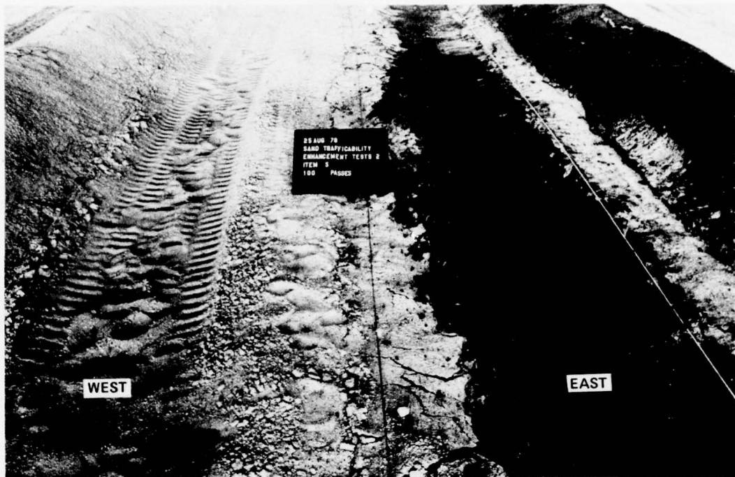
Photo 59. Item 5 after 100 passes, test section 2
