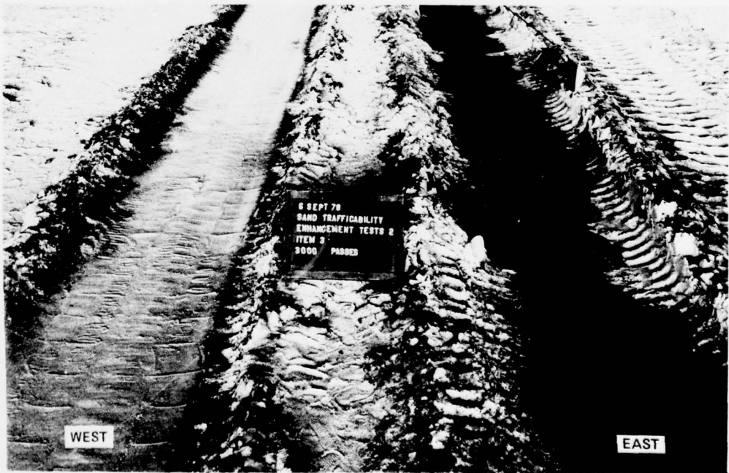
Photo 52. Item 3 after 3000 passes, test section 2
