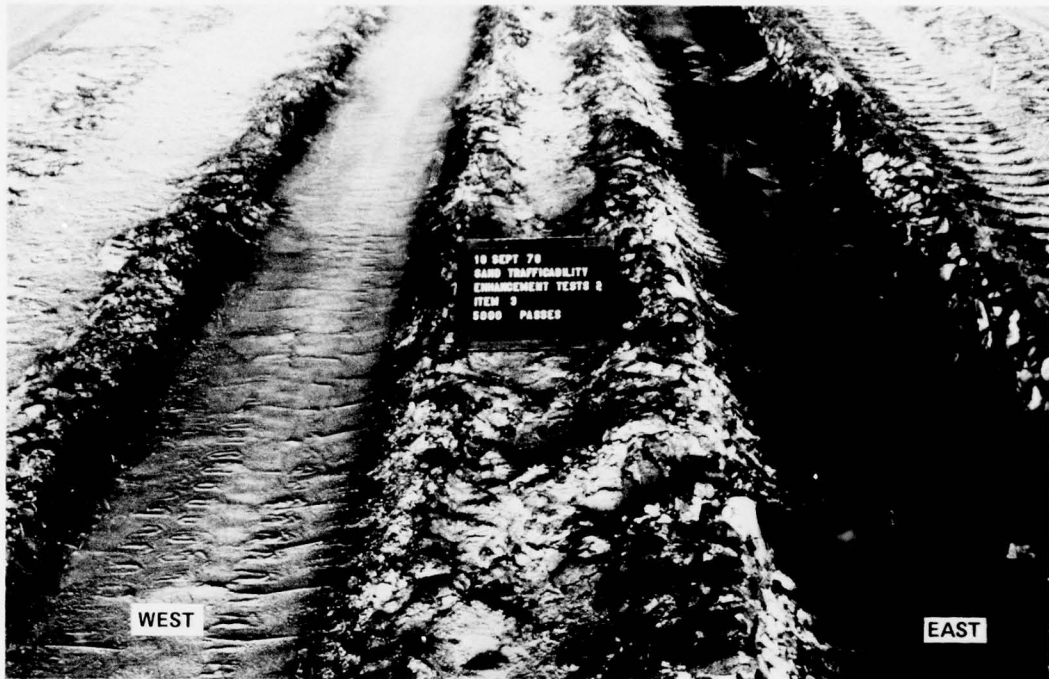
Photo 53. Item 3 after 5000 passes, test section 2
