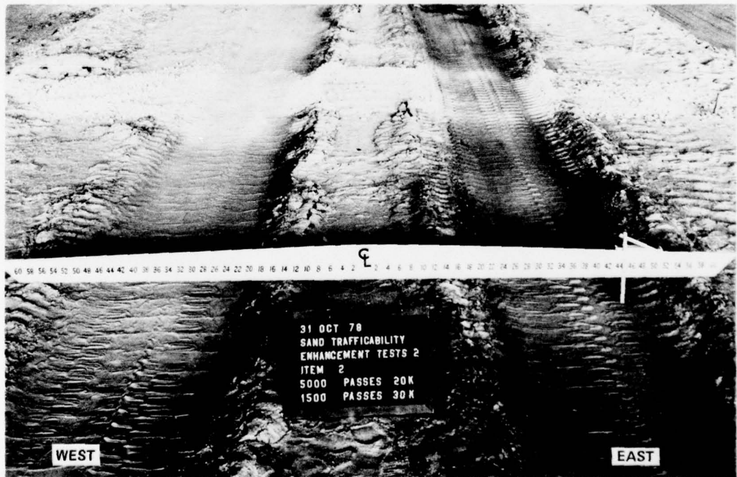
Photo 50. Item 2 after 6500 passes, test section 2
