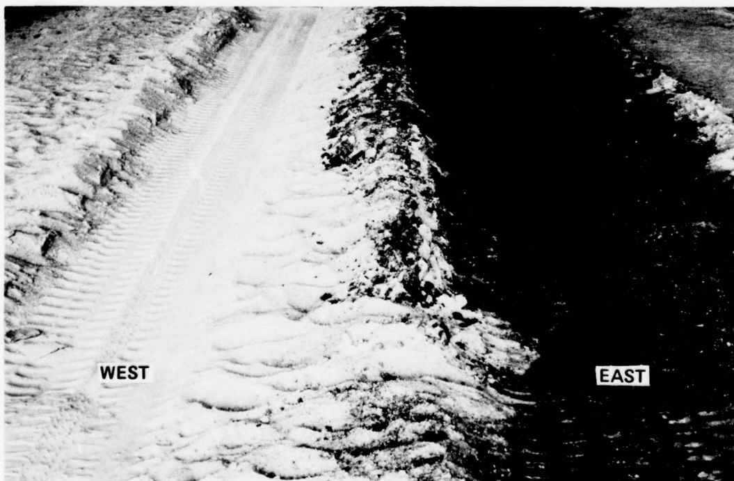
Photo 18. Item 1 after 4850 passes, test section 1
