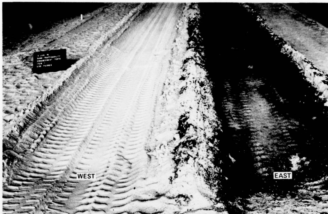
Photo 17. Item 1 after 500 passes of test vehicle, test section 1
