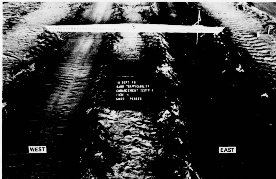
Photo 57. Item 4 after 5000 passes, test section 2
