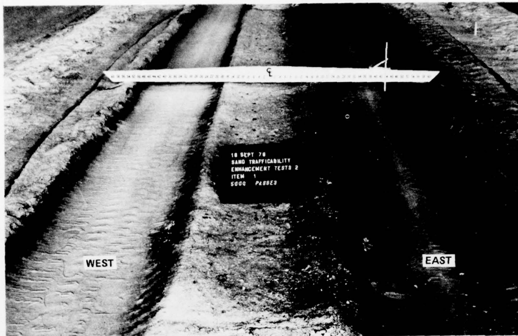
Photo 45. Item 1 after 5000 passes, test section 2
