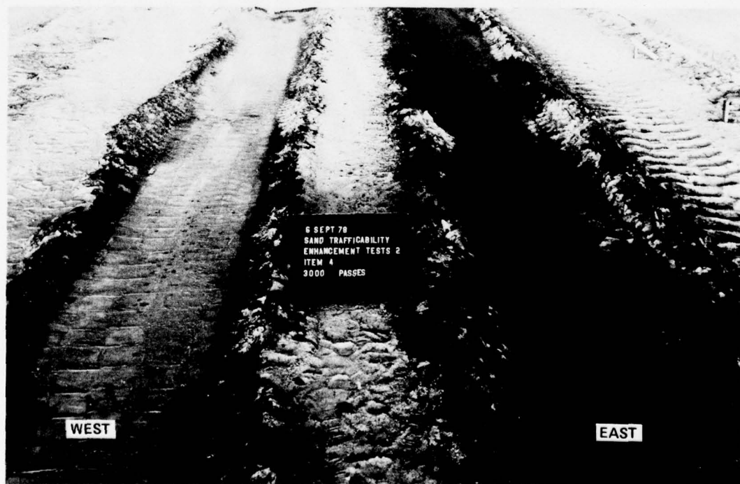
Photo 56. Item 4 after 3000 passes, test section 2
