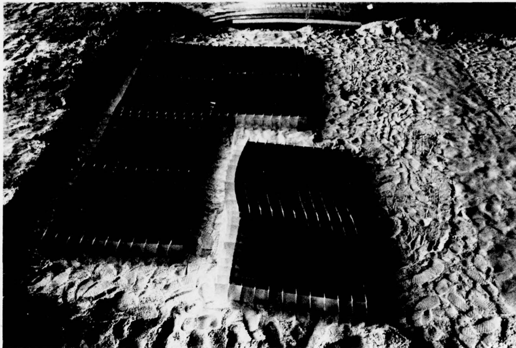
Figure 3. Folded and opened sections of grid
