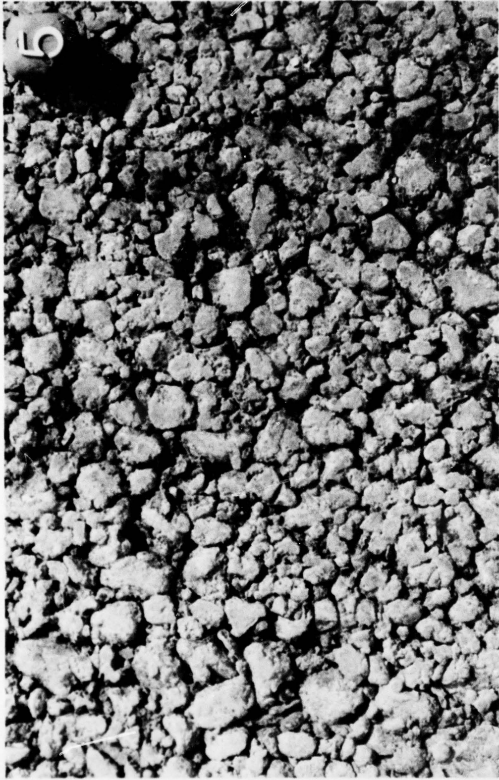
Photo 16. Surface texture of item 5 after compaction
