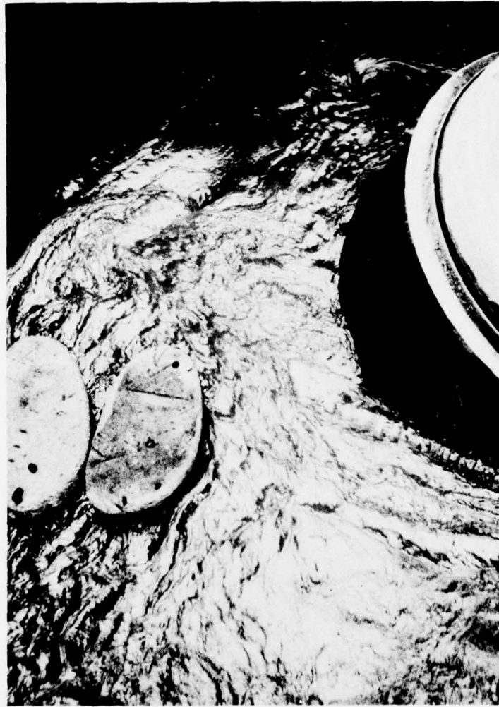
Figure 27. Surface floats to prevent air entrainment in vortexes
