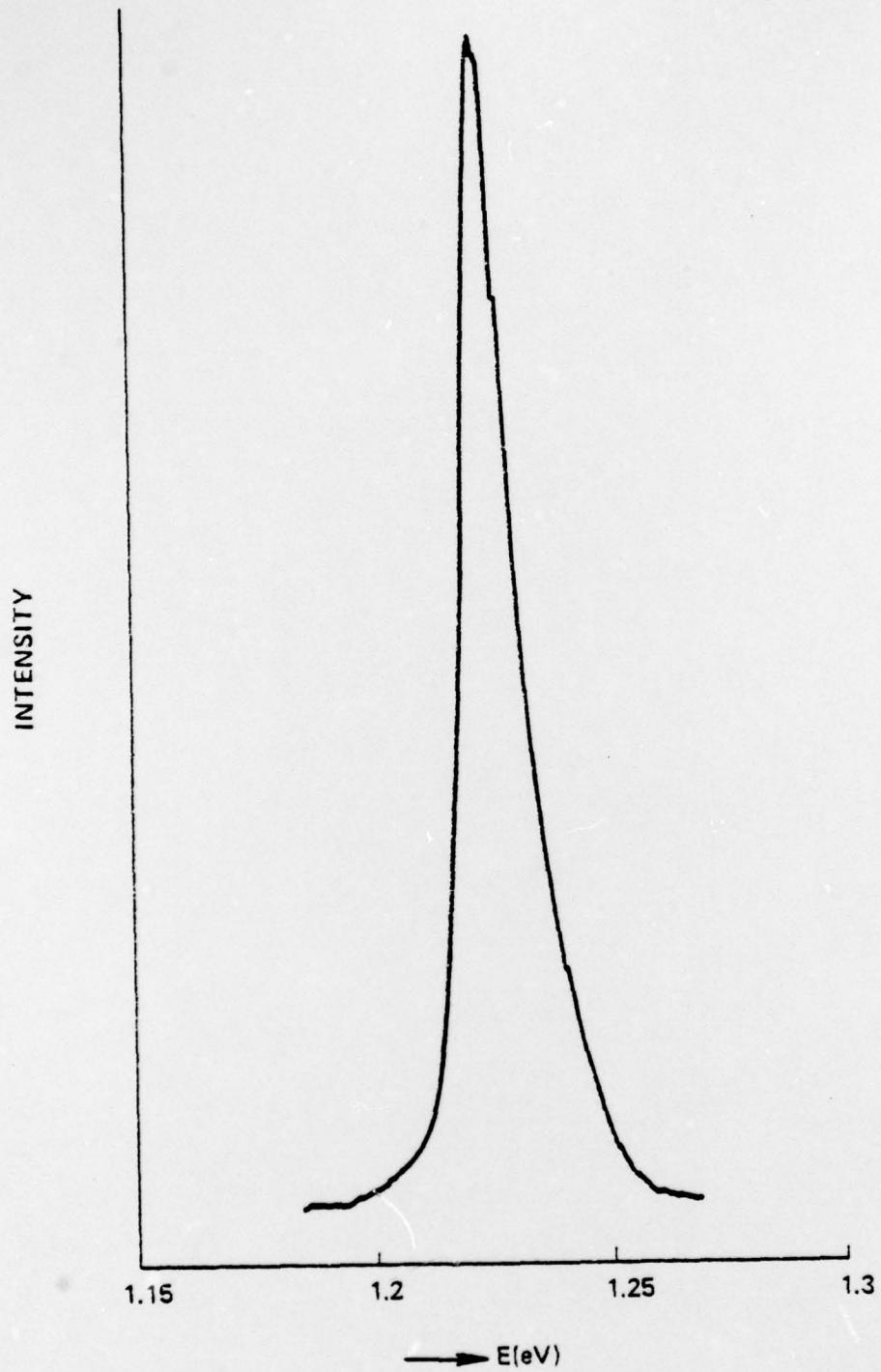
Fig. 4 19% InGaAs photoluminescence spectra
