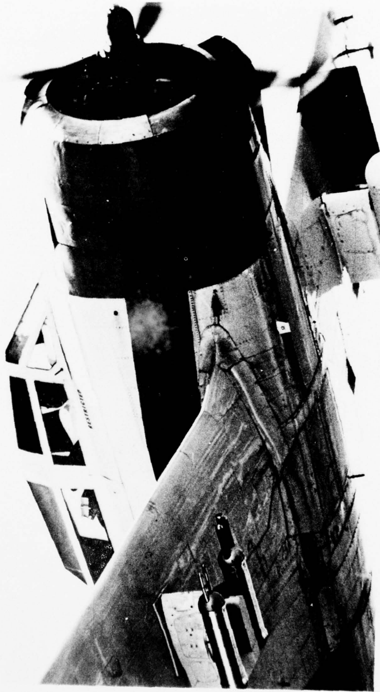
FIGURE 4. T-28 SENSORS WITH THE TOTAL PRESSURE HEADS ON THE LEFT OF THE ANGLE-OF-ATTACK VANE (SMALL POST). (PHOTO BY ROGER ROZELLE--AOPA PILOT MAGAZINE)
