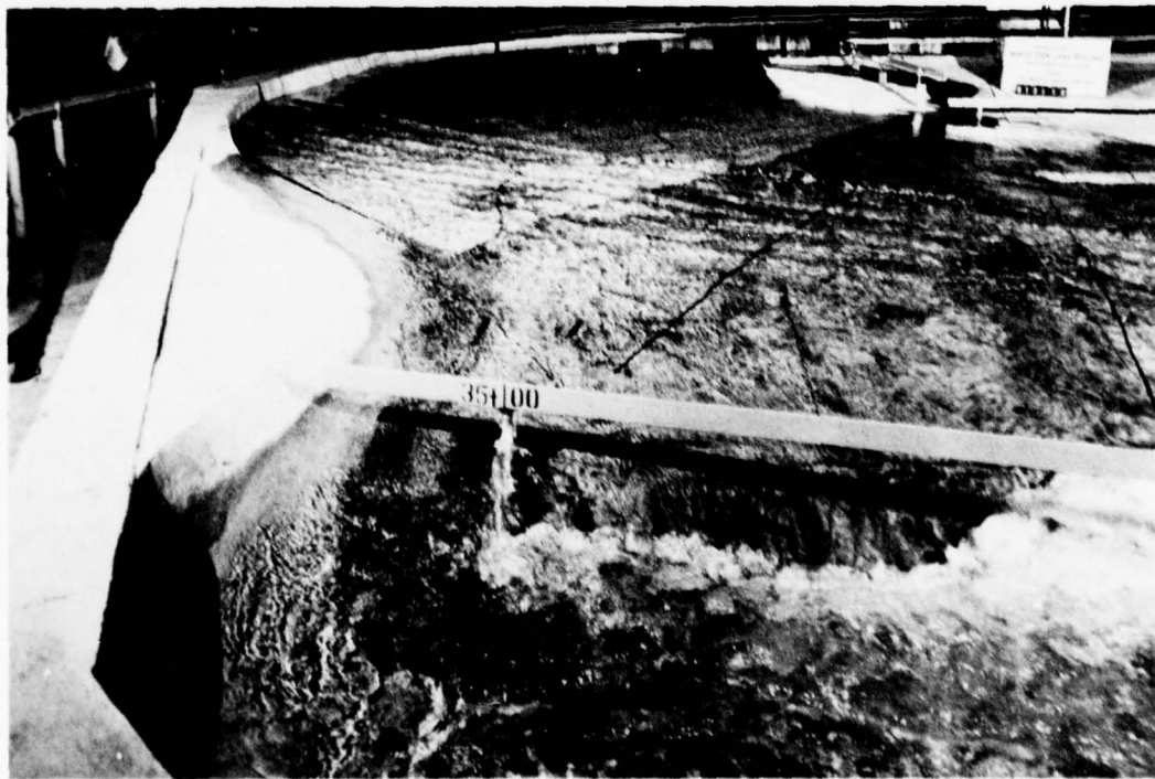
b. Discharge, 284,000 cfs; pool el, 856.6; tailwater el, 752.0
