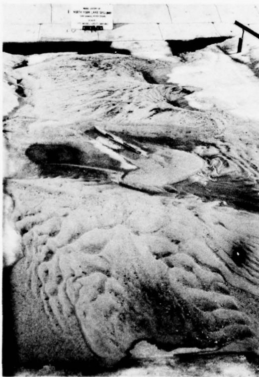
Photo 8. San Gabriel River basin scour resulting from 120-hour hydrograph; peak discharge of 284,000 cfs (8-hr model test duration)
