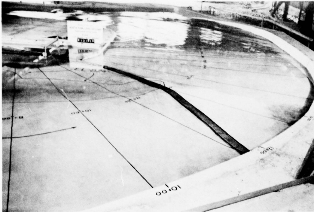
a. Discharge, 88,000 cfs; pool el, 845.0; tailwater el, 731.0
