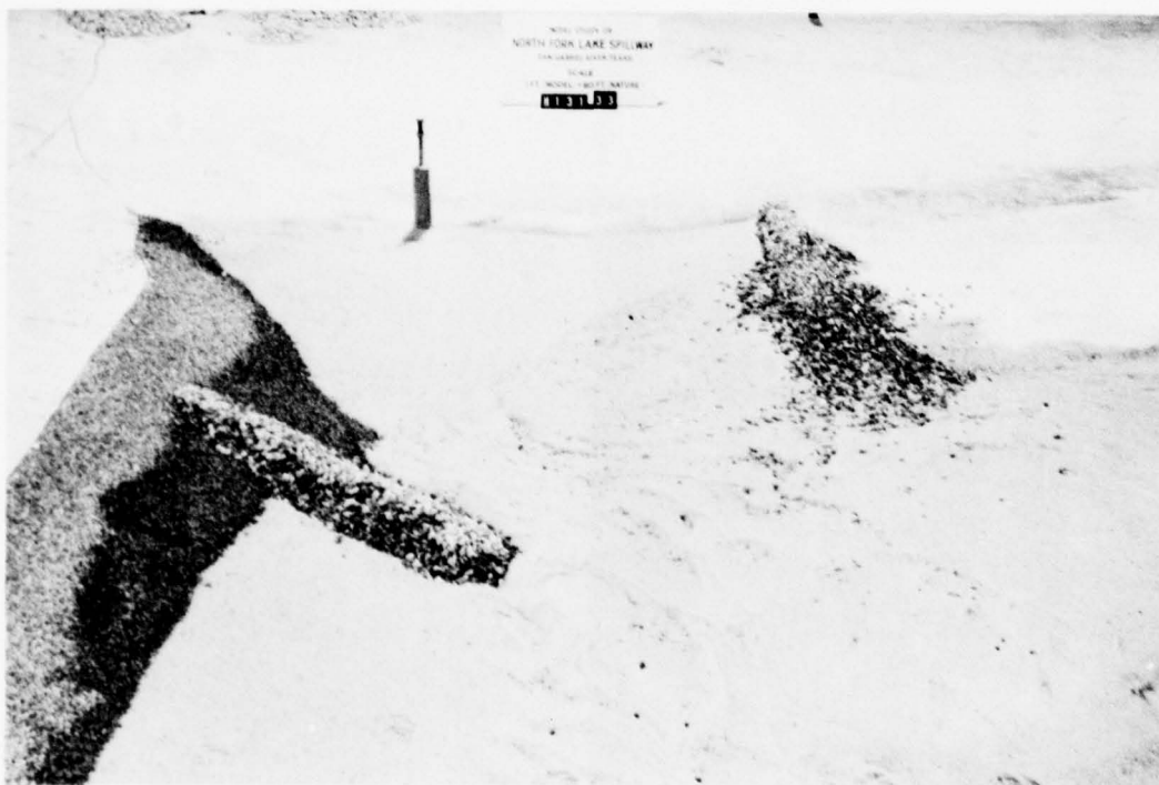
Photo 9. Exit channel and San Gabriel River basin scour with rockfill dikes (type 1 design), rock size d_{50} = 40 in., resulting from 120-hour hydrograph, peak discharge of 284,000 cfs (8-hr model test duration)
