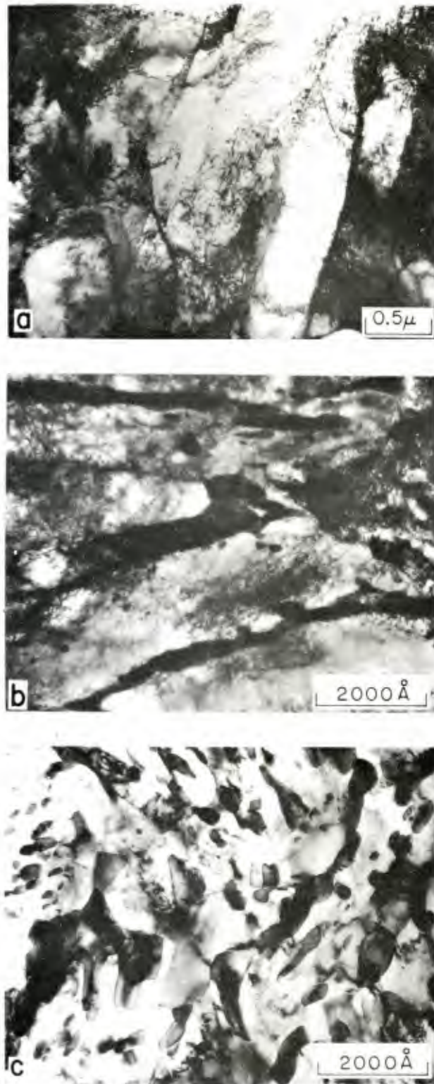
Fig. 14 Transmission electron microscopy of HF-1 steel illustrating (a) the absence of carbide precipitates prior to heat treatment, (b) continuous grain boundary carbide precipitates near the surface following heat treatment and (c) semi-continuous and continuous grain boundary carbide precipitates some distance from the surface.
