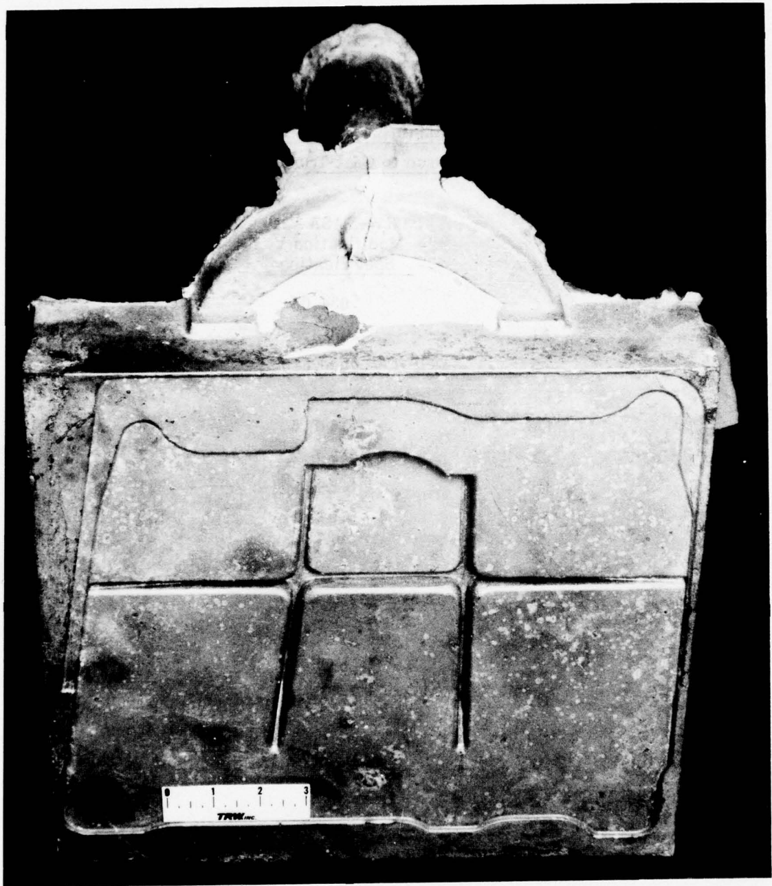
Figure 55. Photograph of trunnion forge tooling showing detail of the as-cast lower die insert configuration.
