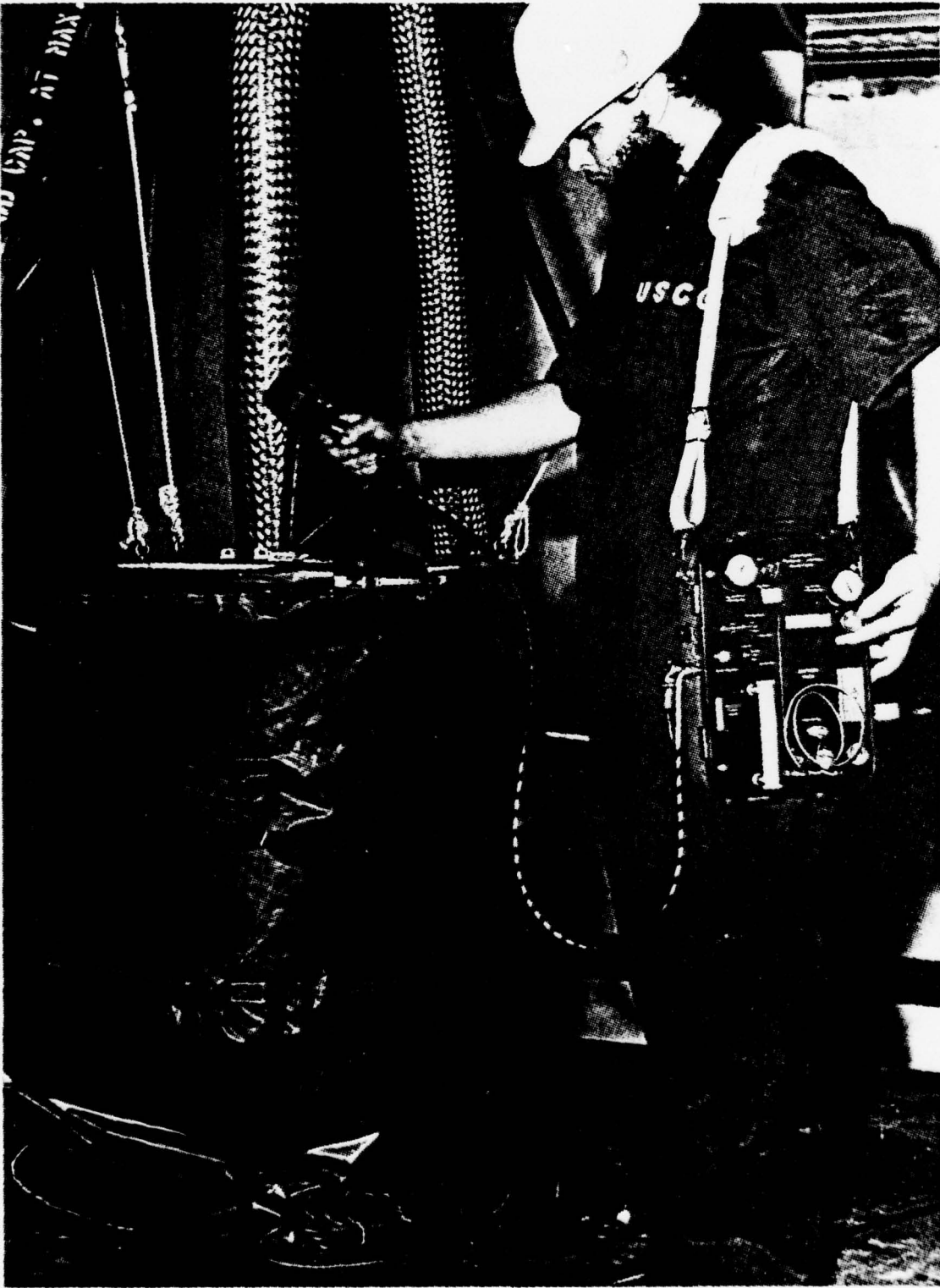
FIGURE 14. VAPOR MEASUREMENT WITH VRD SET IN PLACE FAN IN SECOND POSITION
