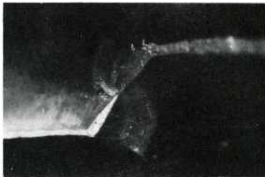
Fig. 23b: BUE Protects the Wear of Lip and Chisel
