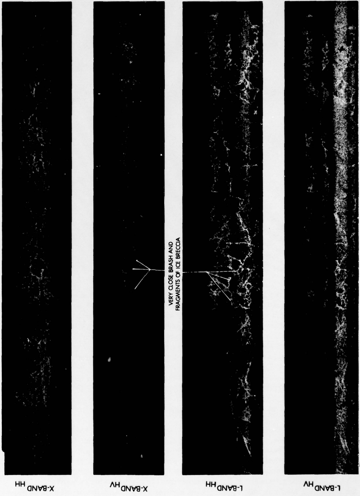
Figure 2. Simultaneous radar images of sea ice off Hopedale Run, Labrador taken by ERIM radar system, 13 March 1977.
