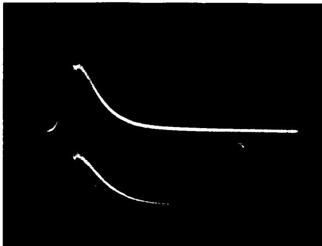
Figure 20. Pump pulse depletion for SRS alone (upper trace) and for simultaneous SRS and SFG (lower trace)
