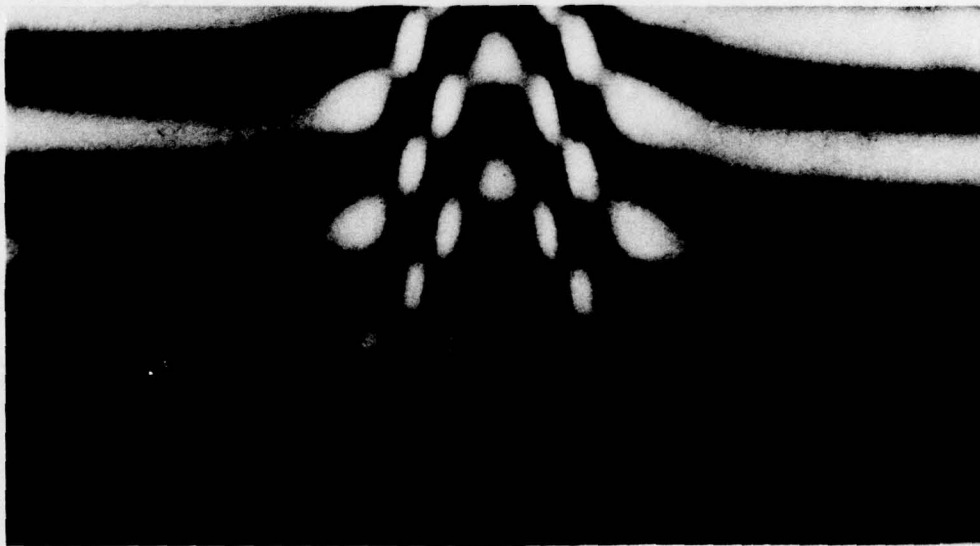
FIGURE 4 - Interference fringes showing the thickness profile fringes due to the groove and perpendicular fringes due to a Michelson interferometric objective.
