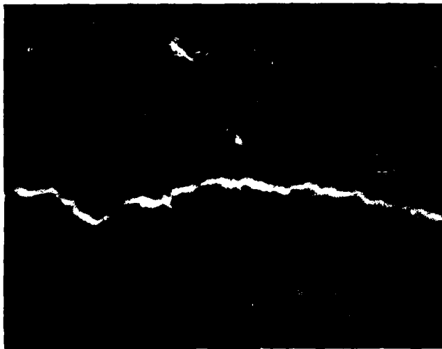
Figure 14. Surface Crack of Rotor Blade 14.
