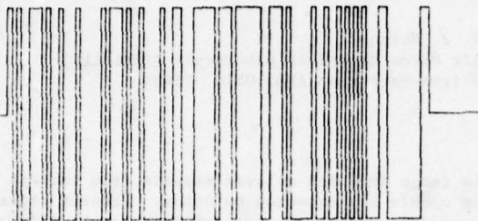
Figure 2. First 100 bits of the pseudorandom binary m-sequence used with the present instrument.
