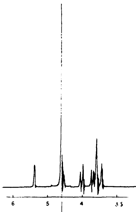
Fig. 4: NMR Spectrum of Authentic Levoglucosan (Solvent: D 2 O Ref: TMS)
