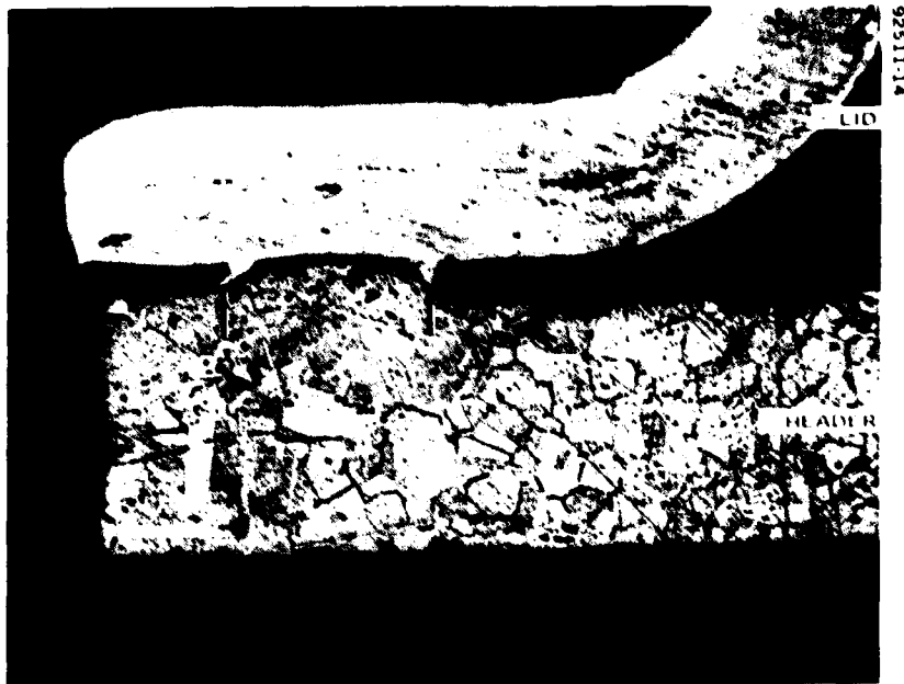
CROSS SECTION OF WELD AREA ON A TF20221 PACKAGE. RAM FORCE = 1600 LBS, HEAT SETTING 95%, TAP 3, HIGH POSITION. 75X.
