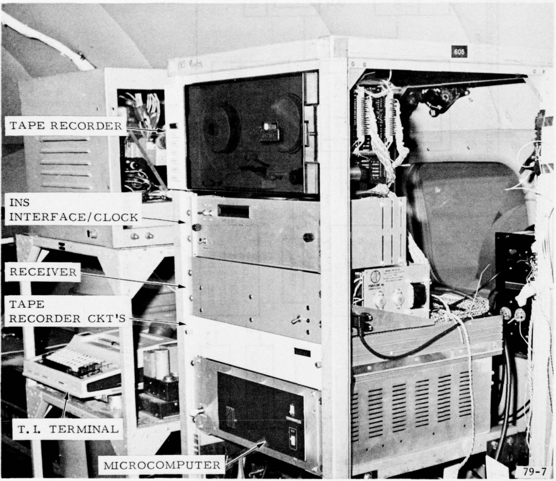
FIGURE 2. ITS DATA RECORDING SYSTEM
